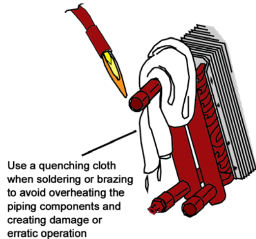
Figure 7: Protect Components From Overheating
