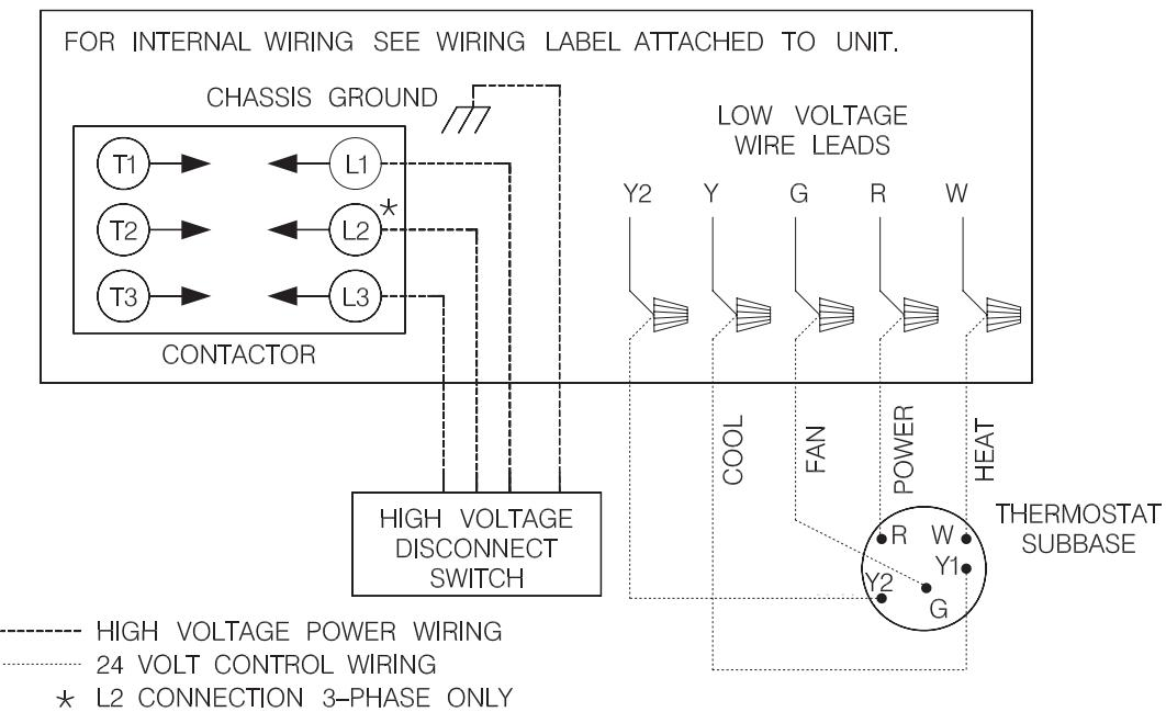
**Figure 16: Optional Factory Supplied 7-170 Thermostat Wiring Diagram**
