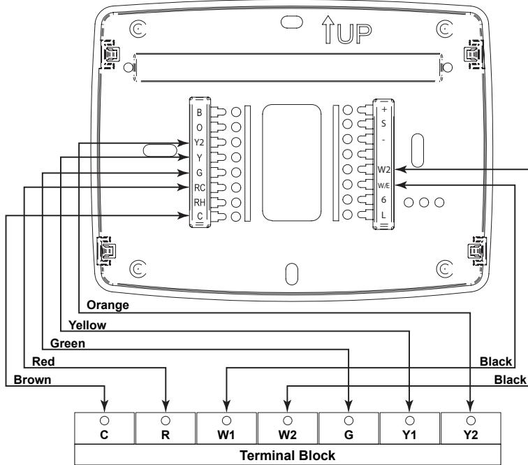
1. On 3 to 5 ton units, a terminal block is not supplied. Use a wirenut to extend from the leads provided in the unit to the thermostat. W1, W2, and Y2 are optional depending upon the size and selected options of the unit. Colors shown above are typical for the MPS I.
