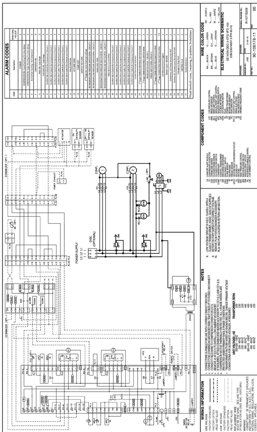
**Figure 21: MPS 007-010D, 208-230/460 Volt (Two-Speed SAF Gas Heat — DDC Controls)**
