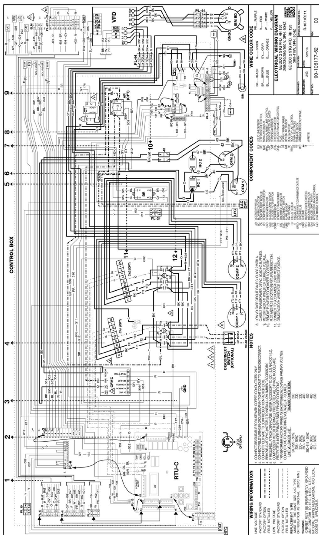
**Figure 34 continued: MPS 012D, 208-230/460 Volt (Two-Speed SAF with HGRH — DDC Controls)**
