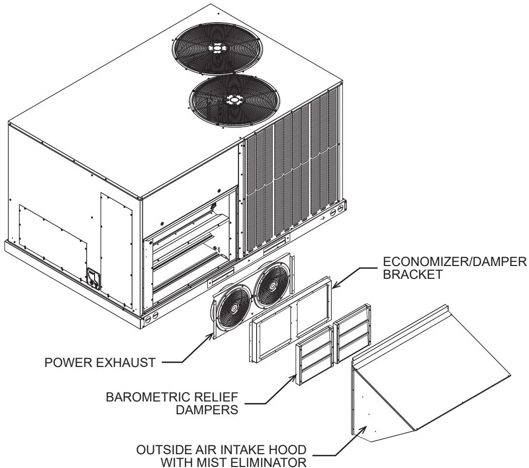
**Figure 51: Horizontal Airflow Power Exhaust Economizer, MPS 007D – 012D**
