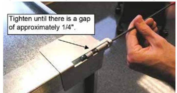
Figure 24: Tighten Cap Screw to 1/4" of the Coupling
