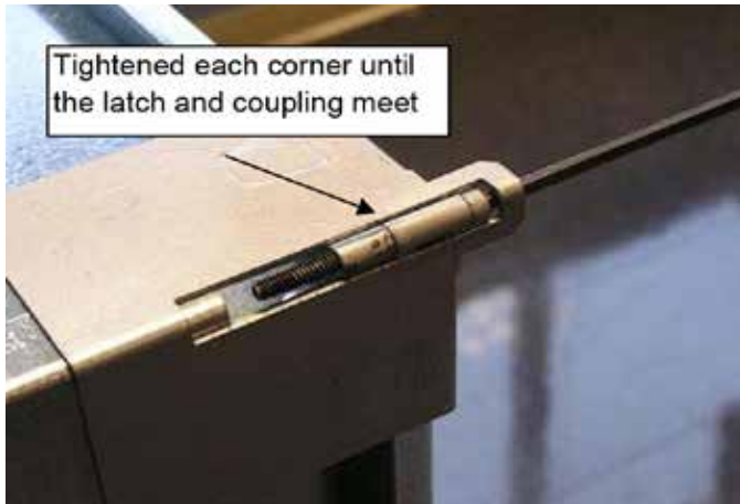
Figure 25: Tighten until Latch and Coupling Meet
