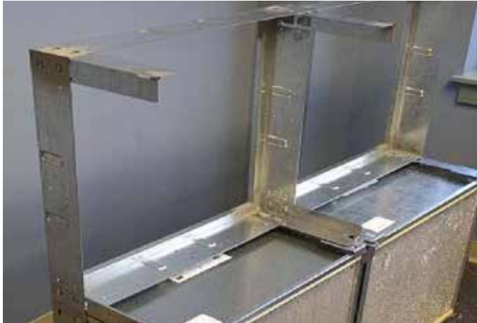
Figure 20: Frame with Leg Extensions Installed
