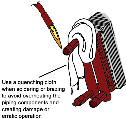
Figure 6: Protect Components from Overheating
