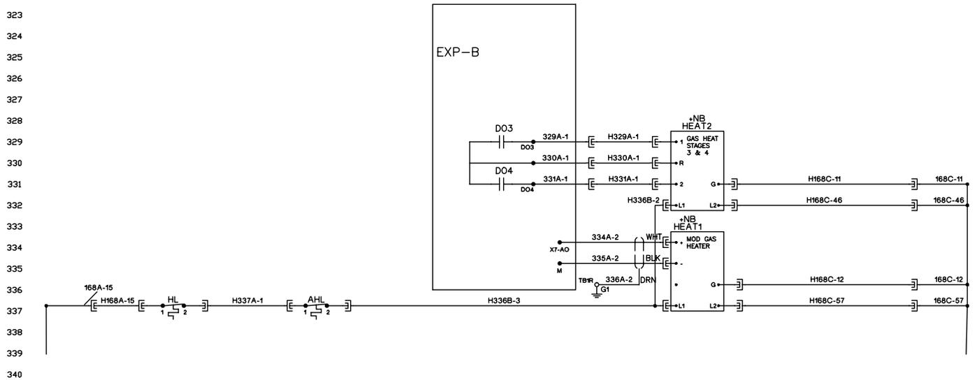
**Figure 74: Electric Heat Option Power**
