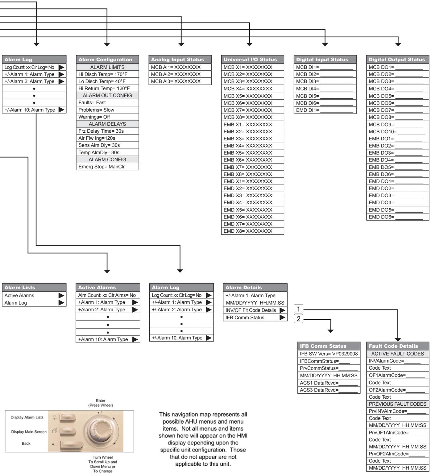
**Figure 100: BMS Communications – Keypad/Display Menu Structure**
