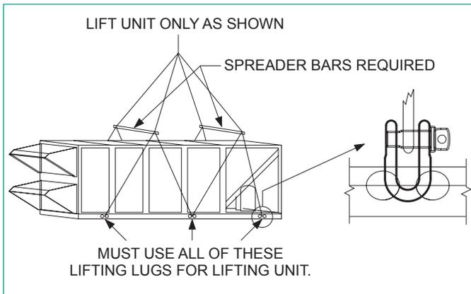
Use spreader bars, 96" to 100" (2438 to 2540 mm) wide to prevent damage to the unit cabinet. Avoid twisting or uneven lifting of the unit. The cable length from the bracket to the hook should always be longer than the distance between the outer lifting points.
