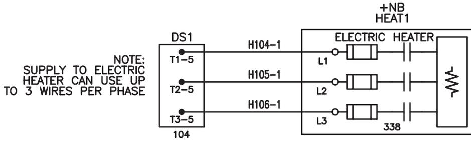
**Figure 75: Electric Heat Option – Outputs**
