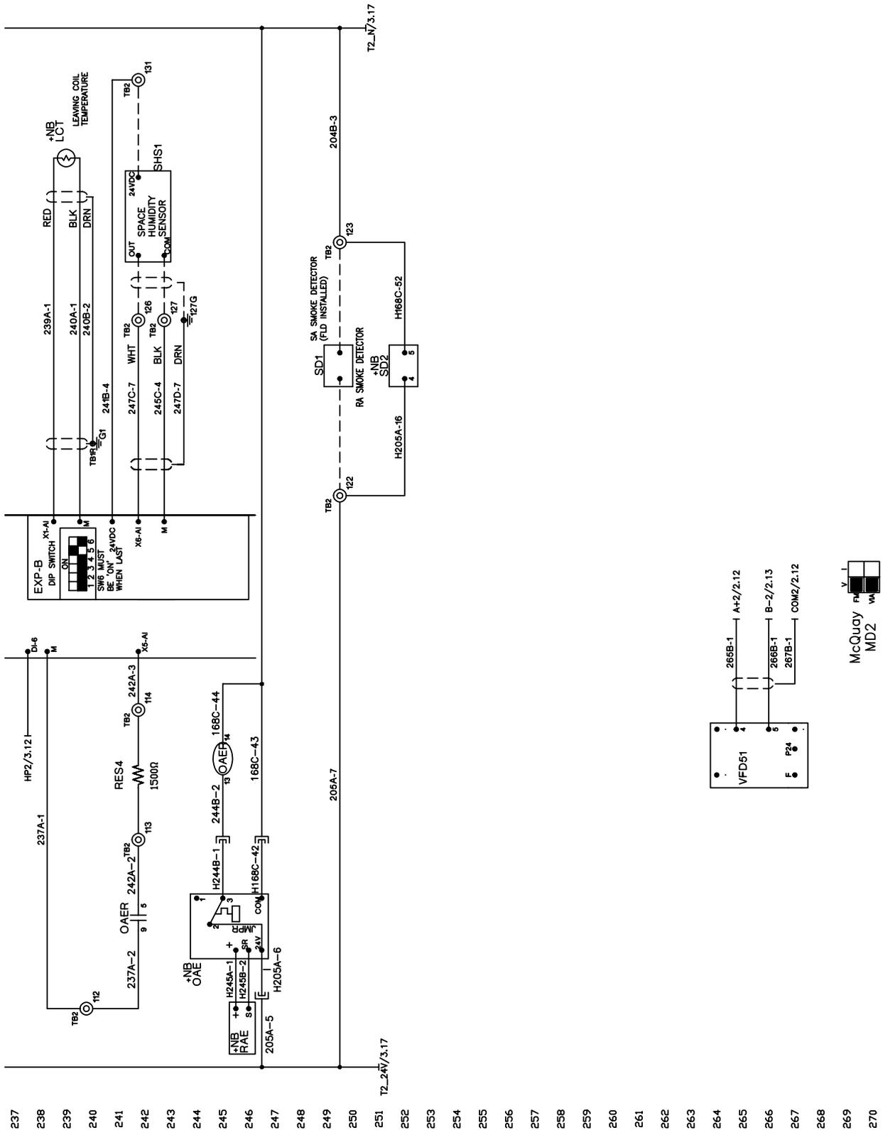
Figure 72: CAV Control – Outputs (Staged Gas Heat)
