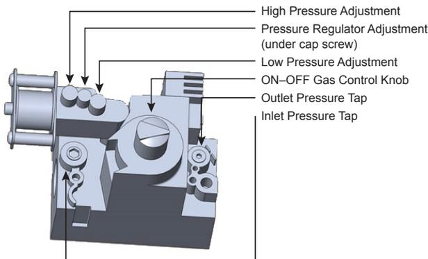
**Figure 26: Maxitrol M520B Modulating Valve**
