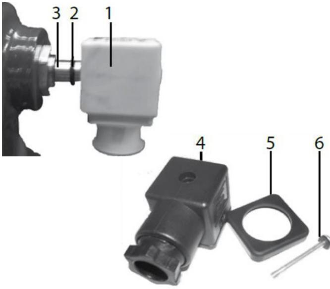
Figure 58: Oil Injection Control Dismantling
