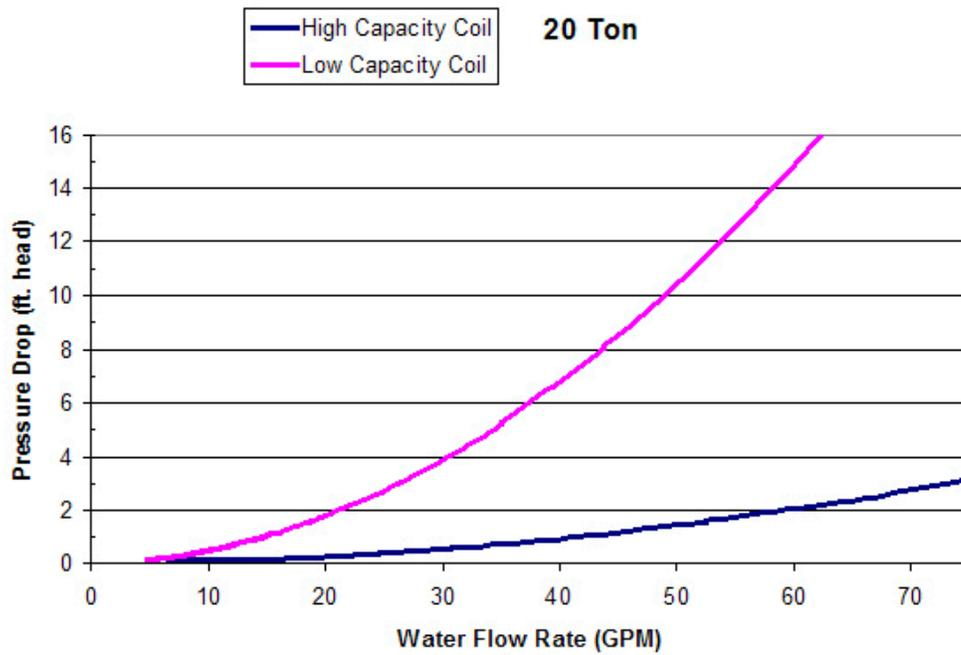
Figure 39: MPS 026 – 035 Low and High Heat
