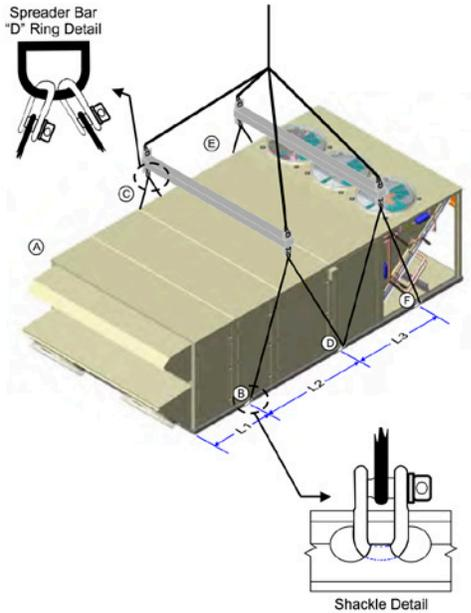
Figure 11: Rigging the Unit (MPS 040–050 Example)
