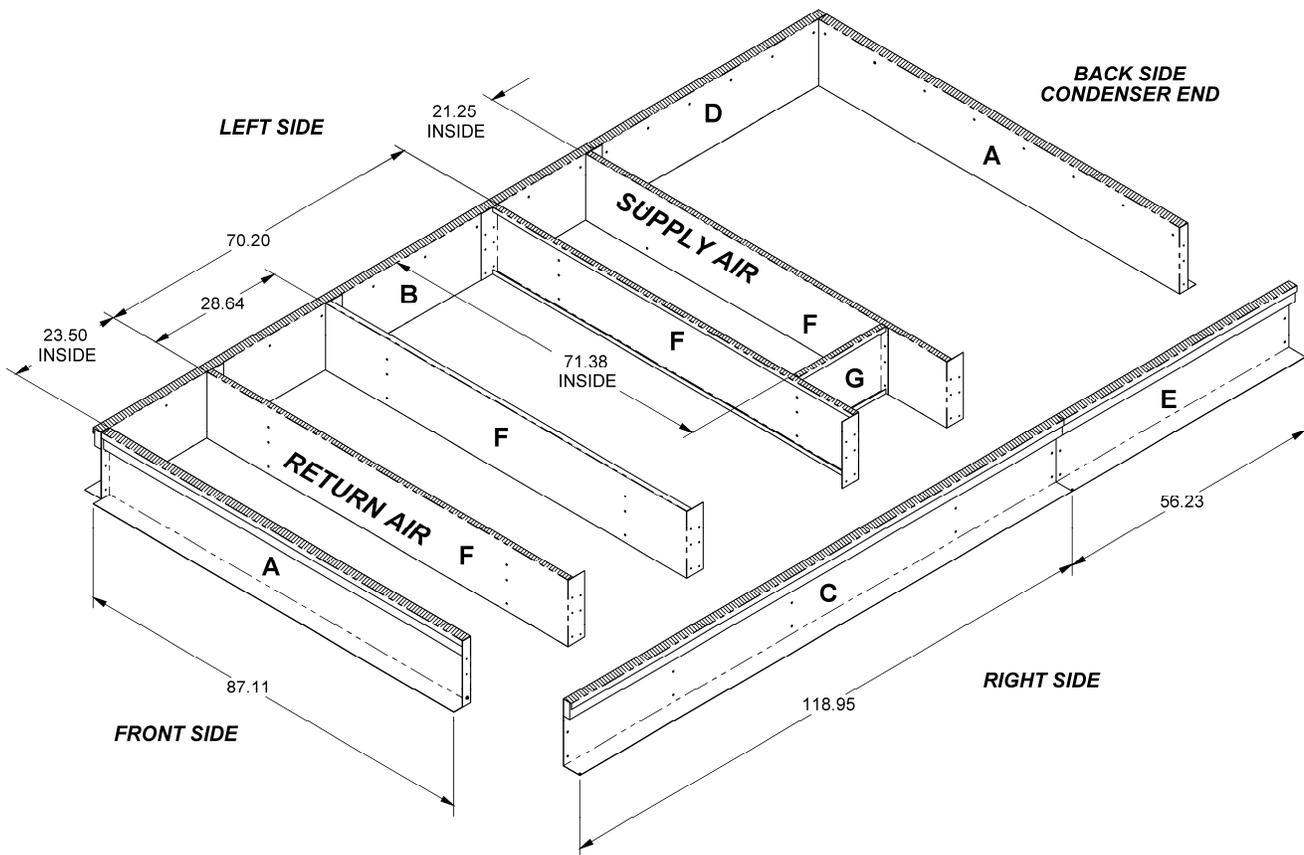
**Figure 3: Roof Curb Layout—MPS 015F – 020G**
