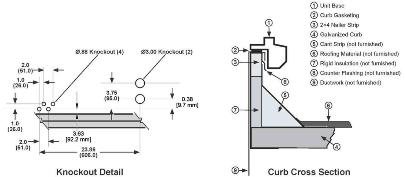
Figure 8: MPS 040–050 Roof Curb with Energy Recovery Wheel
