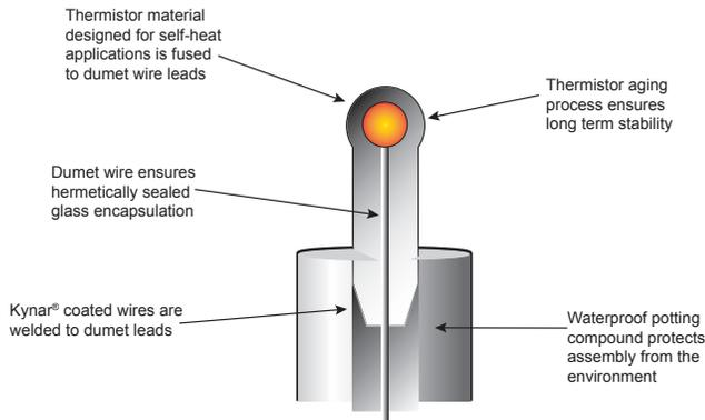
**Figure 46: Bead-in-Glass Thermistor Probe**
