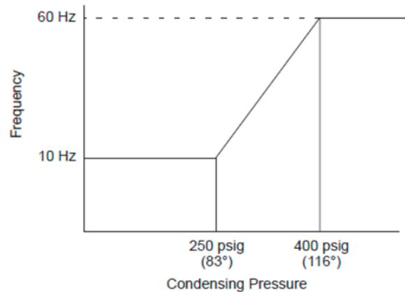
Figure 53: Speedtrol Operating Characteristics (for Variable Speed Inverter Compressor Units with Start-Stop Control)
