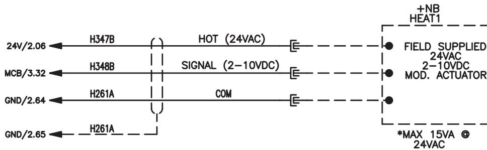
Figure 36: Hot Water Heat Vestibule
