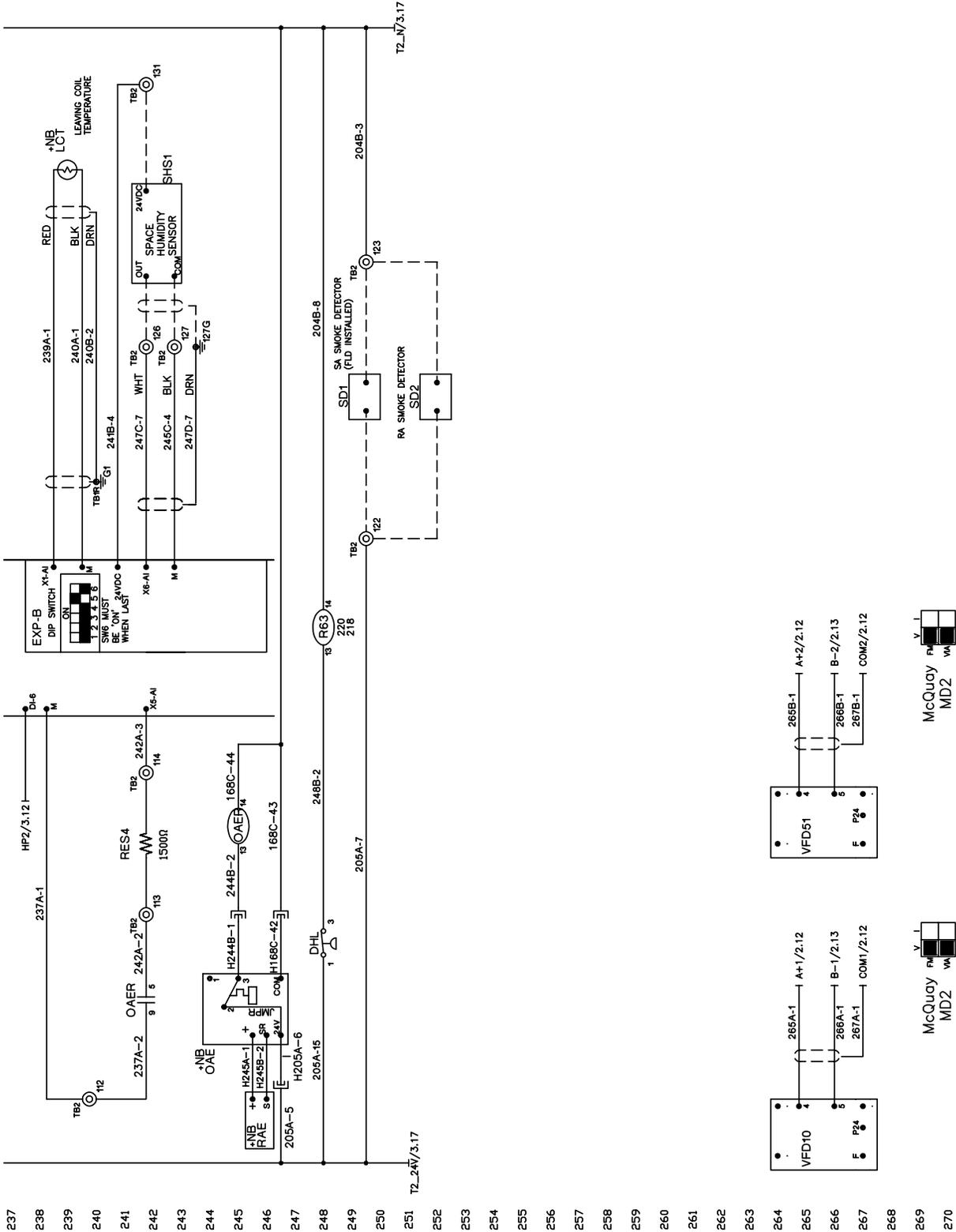
Figure 65: MPS 026 VAV Control with Variable Speed Inverter Compressor
