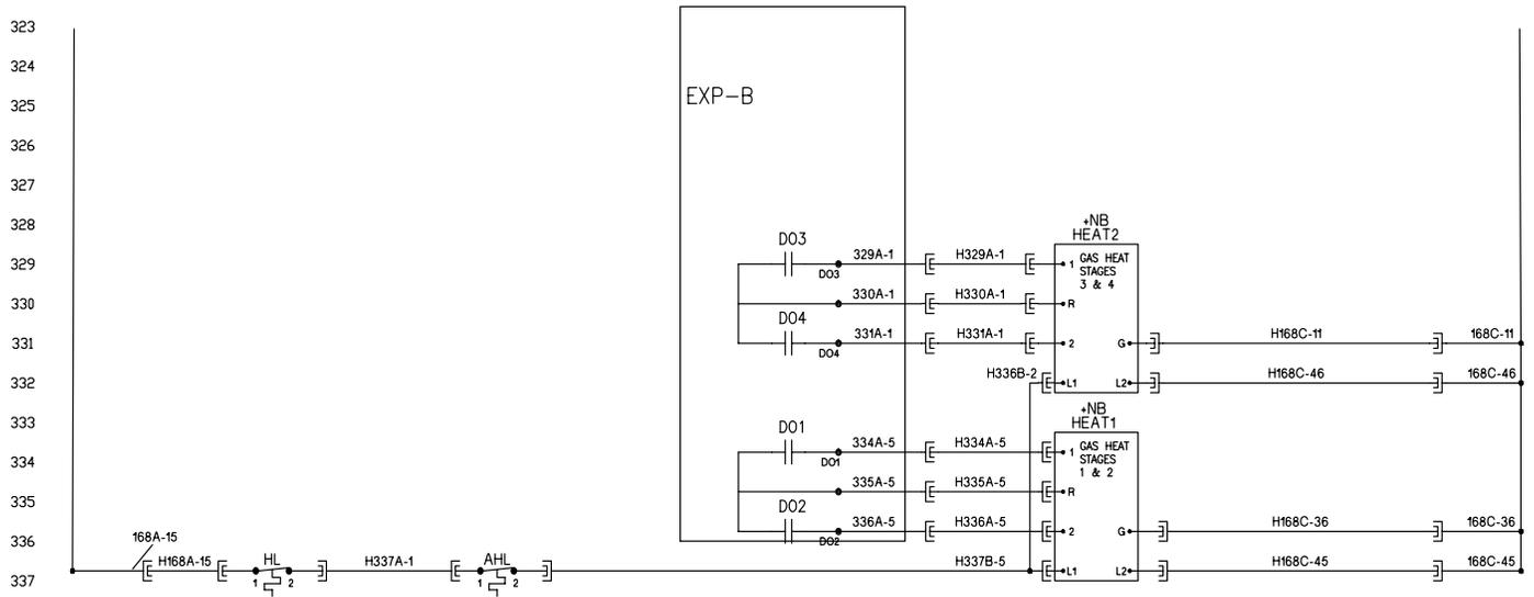
Figure 73: VAV/CAV Control – Outputs (Modulating Gas Heat)
