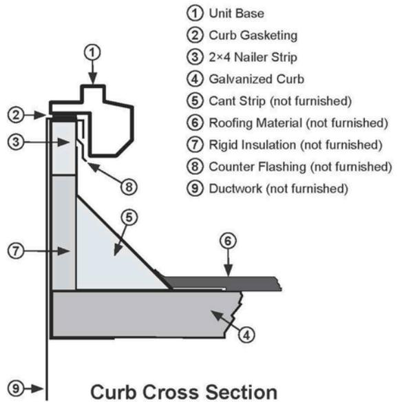
Figure 7: MPS 026–035 Roof Curb with Energy Recovery Wheel
