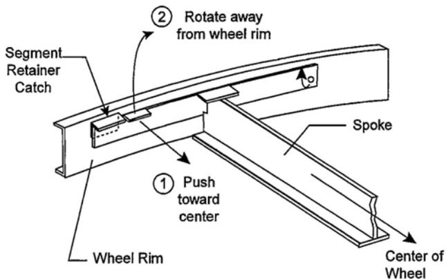
Figure 92: Installing Wheel Segments
