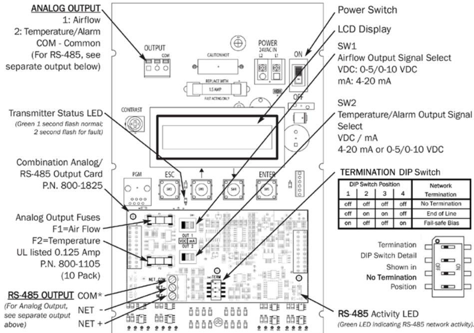
Figure 48: Transmitter and Connector Detail
