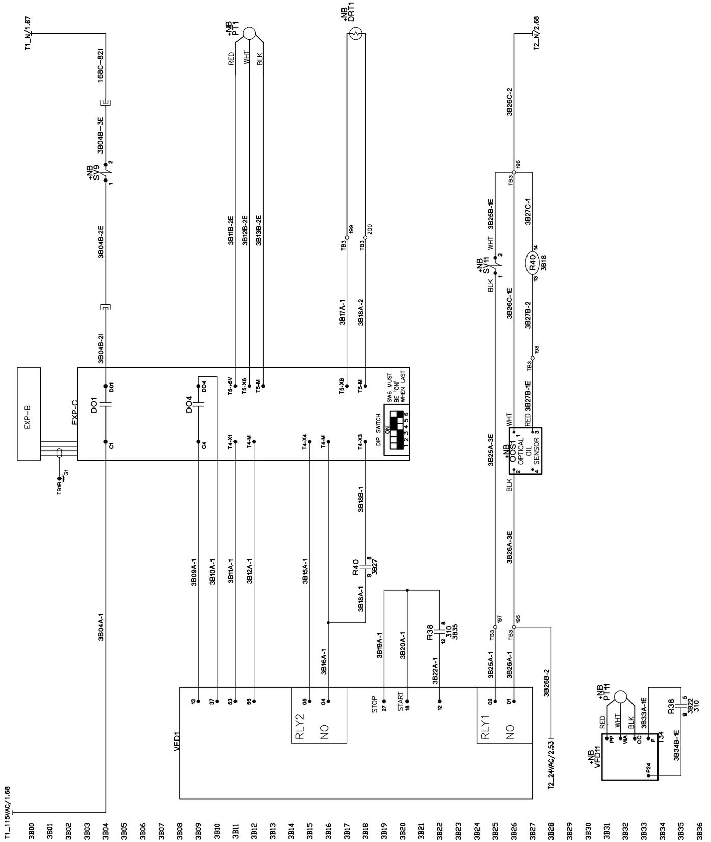
Figure 69: VAV Control – Outputs (Staged Gas Heat)
