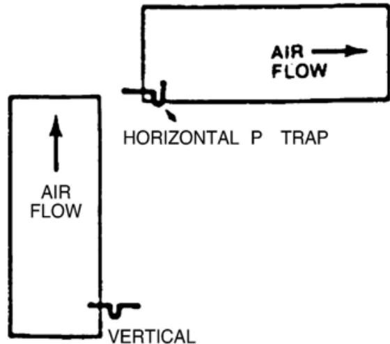
Figure 13: Coil Above Condensing Unit
