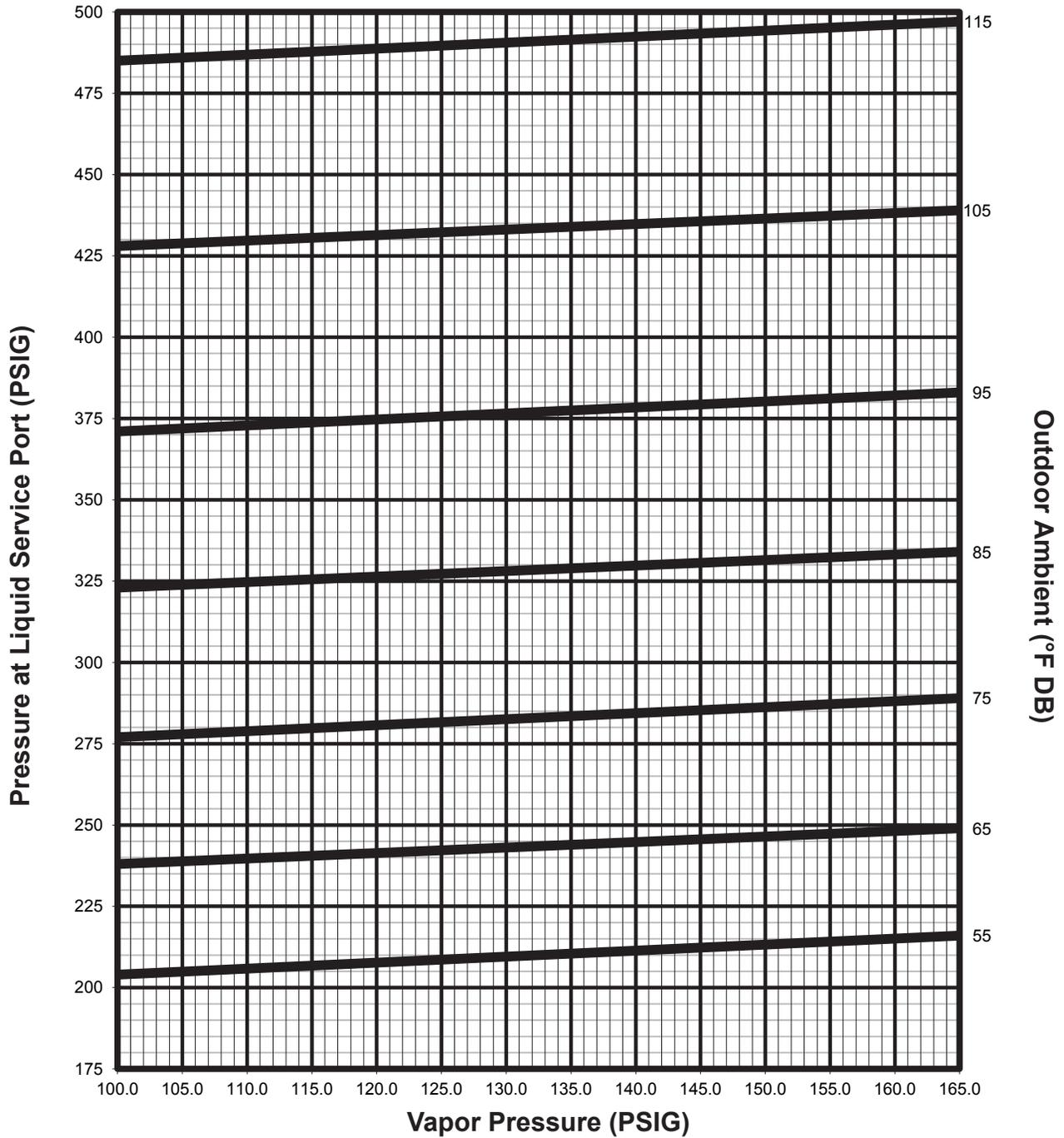
**CAUTION: RETURN AIR TEMPERATURE MUST BE WITHIN COMFORT CONDITIONS BEFORE FINAL REFRIGERANT CHECK!**
