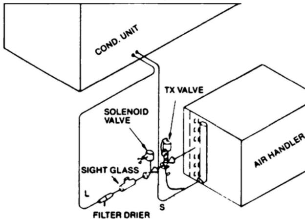
NOTE: PIPING ACCESSORIES SHOWN SHOULD BE MOUNTED AS CLOSE TO AIR HANDLER AS POSSIBLE.
