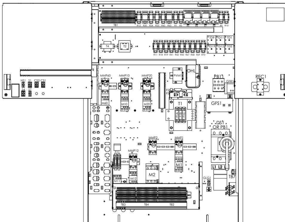
**Figure 13: Typical Main Control Panel, 036C - 040C, 208 Volt**
