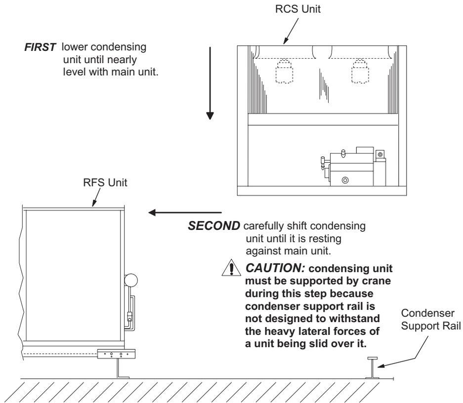
**Figure 50: Caulk and Install Parts, Steps 10–14**
