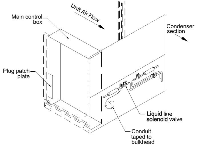
**Figure 55: Remove Vertical Raceway**
