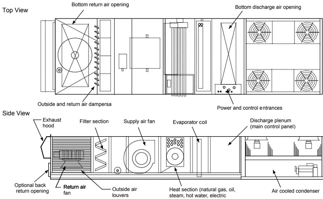
**Figure 4: Component Locations—RDT Units**
