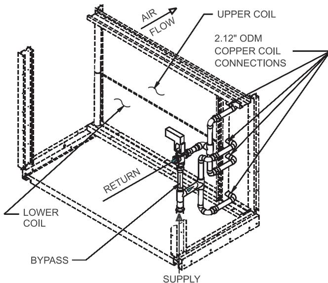
**Figure 58: Hot Water Valve Package**
