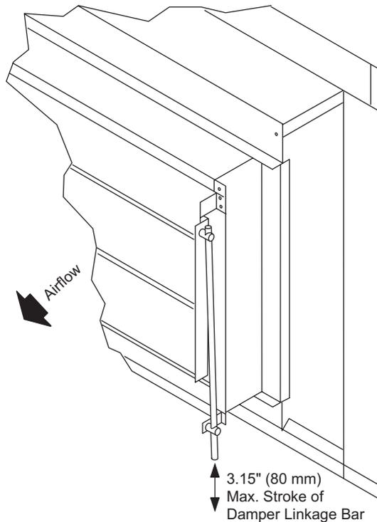
**Figure 63: Intake Hood Damper Adjustment**
