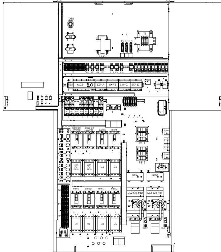
**Figure 16: Typical Gas Heat Panel, 1000 MBH**
