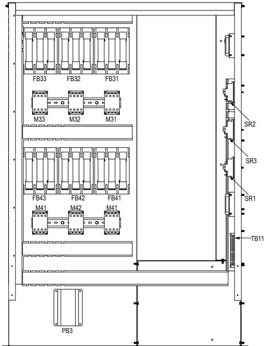
**Figure 24: Electric Heat Panel, Sizes 080C - 105C**
