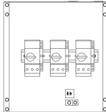
**Figure 18: Figure 18: VFD Bypass Panel, 40 HP, 460 Volt**
