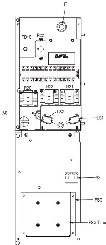
**Figure 17: Typical Prop Exhaust Panel, 3 Fans, 460 Volt**
