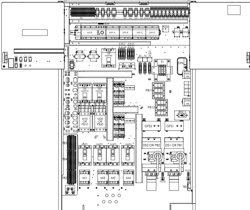
**Figure 15: Typical Main Control Panel, 080C - 105C, 460 Volt**
