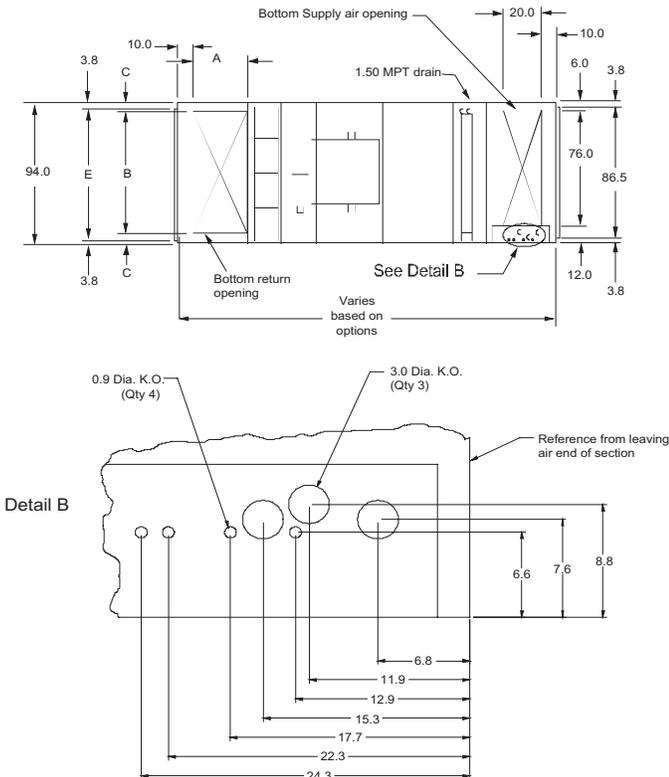
**Figure 70: RCS 015C - 030C Power Wiring Connections**
