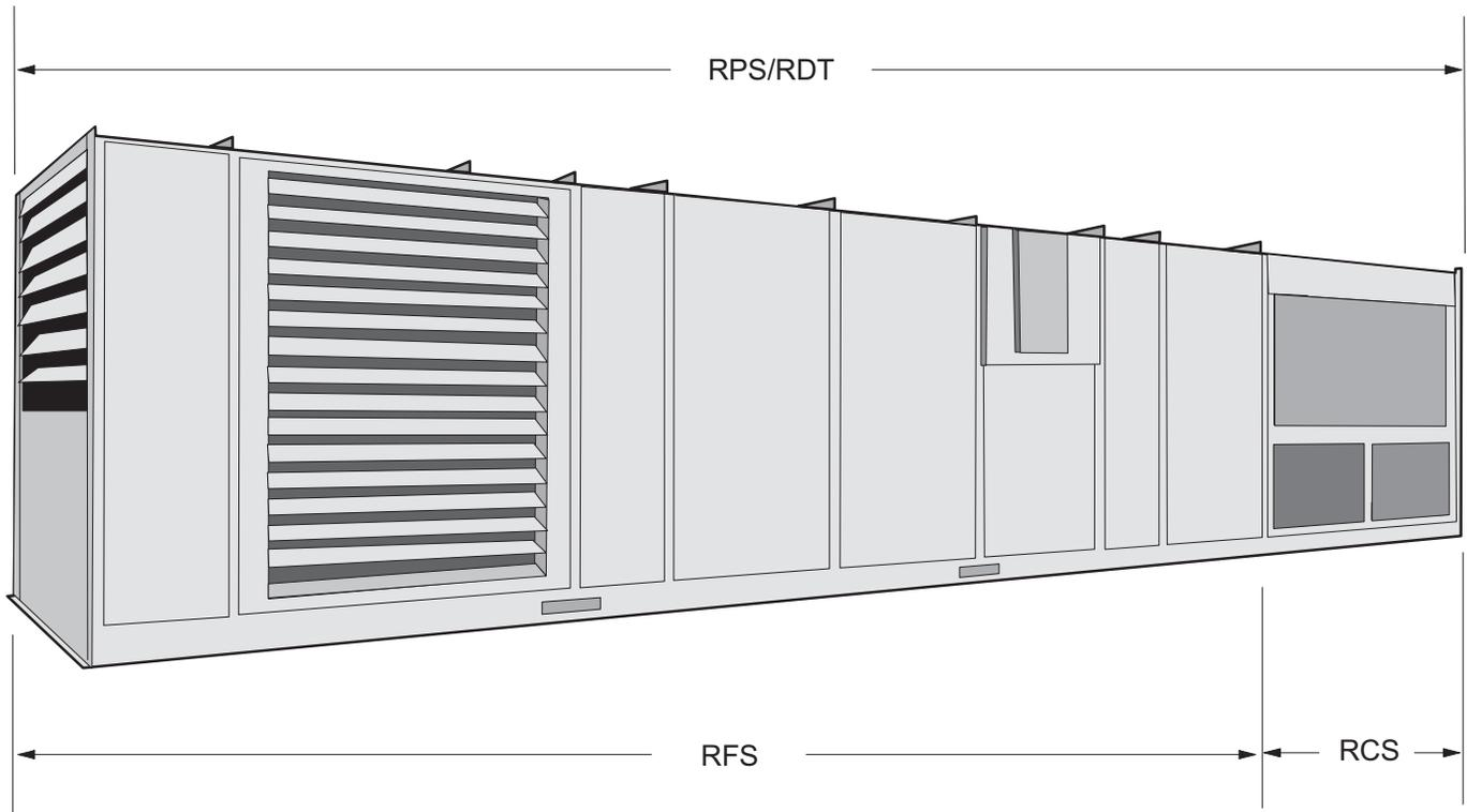
**Figure 3: Typical Component Locations—RPS Units**
