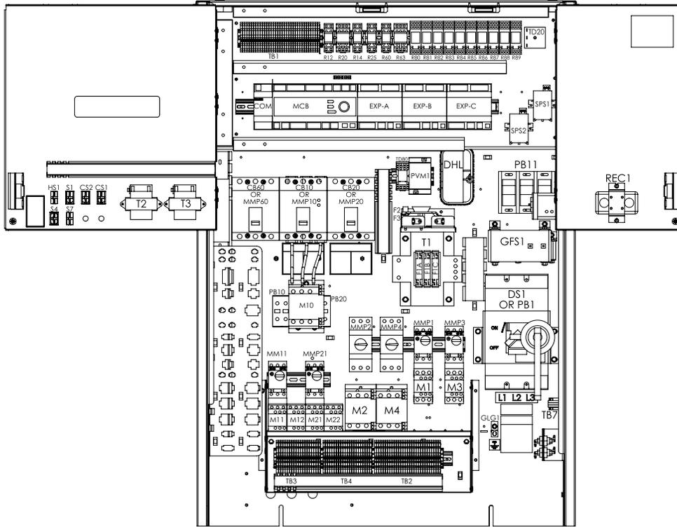
**Figure 14: Typical Main Control Panel, 045C - 075C, 460 Volt**
