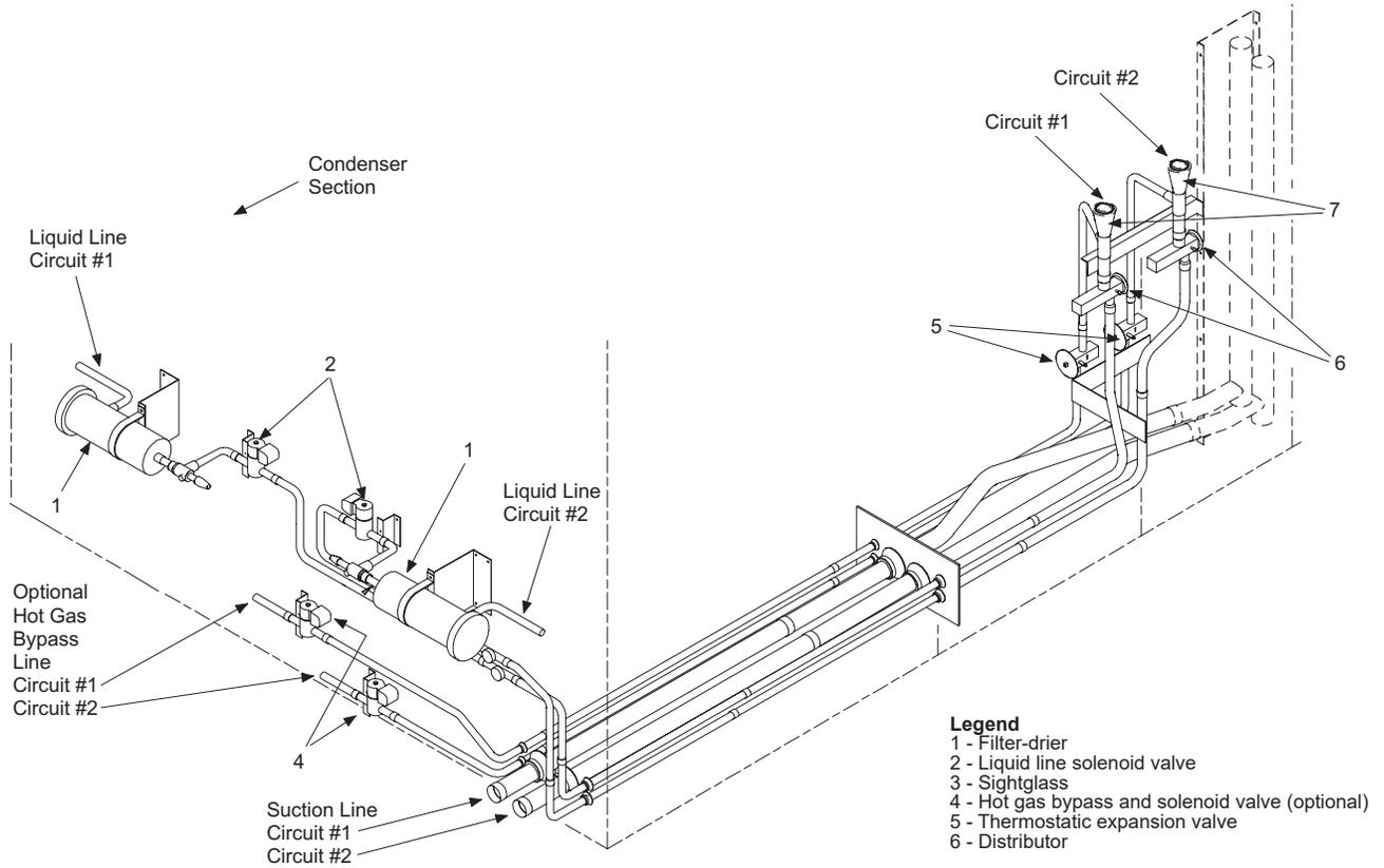
**Figure 8: Air Handler Piping (Staggered DX)**
