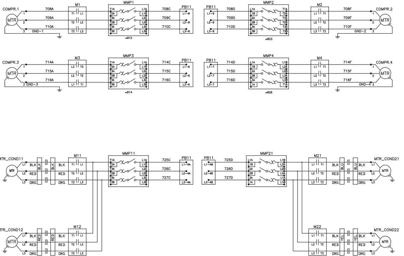
Figure 87: VFD Control (SAF and RAF)
