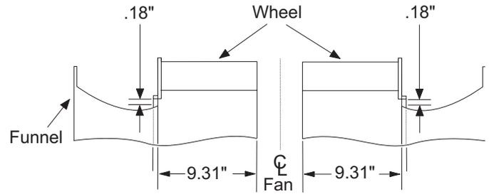
**Figure 124: 27" to 40" DWDI Airfoil Wheel-to-Funnel Alignment**
