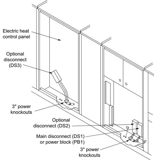
**Figure 68: Optional Side Power Wiring Entrance**
