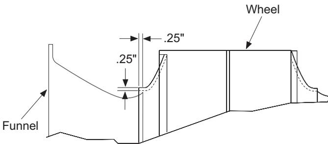
**Figure 123: 24" DWDI Backward Curved Wheel-to-Funnel (036C, 040C)**
