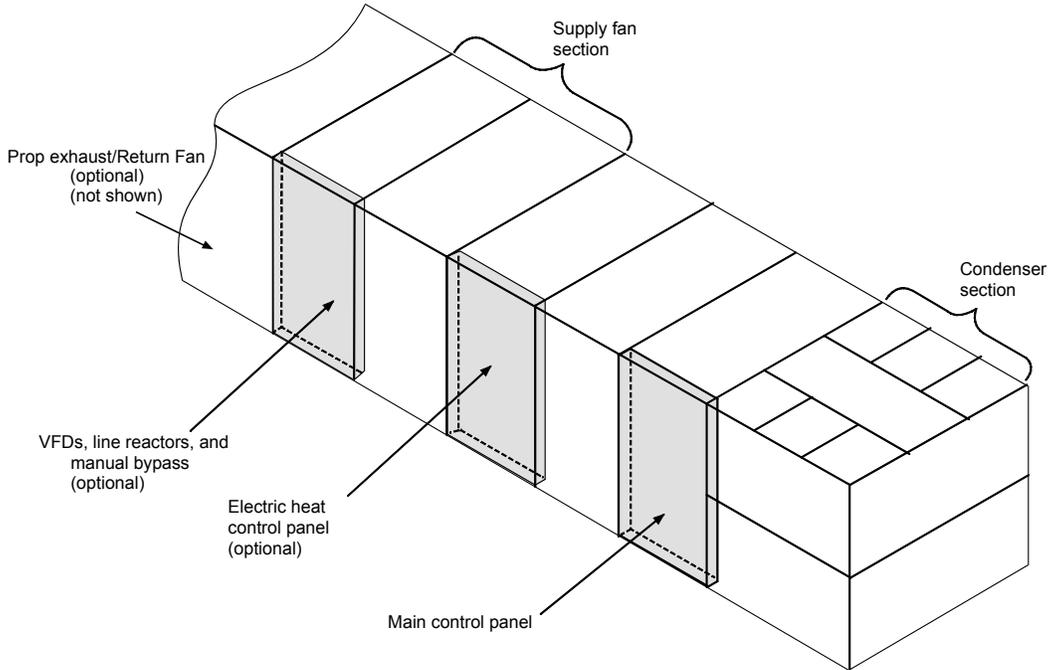
**Figure 12: Typical Main Control Panel, 015C - 030C, 460 Volt**
