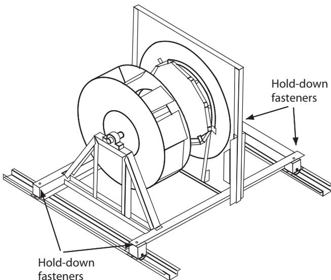
Figure 76: Spring Mounted Hold-Down Fasteners, All Units
