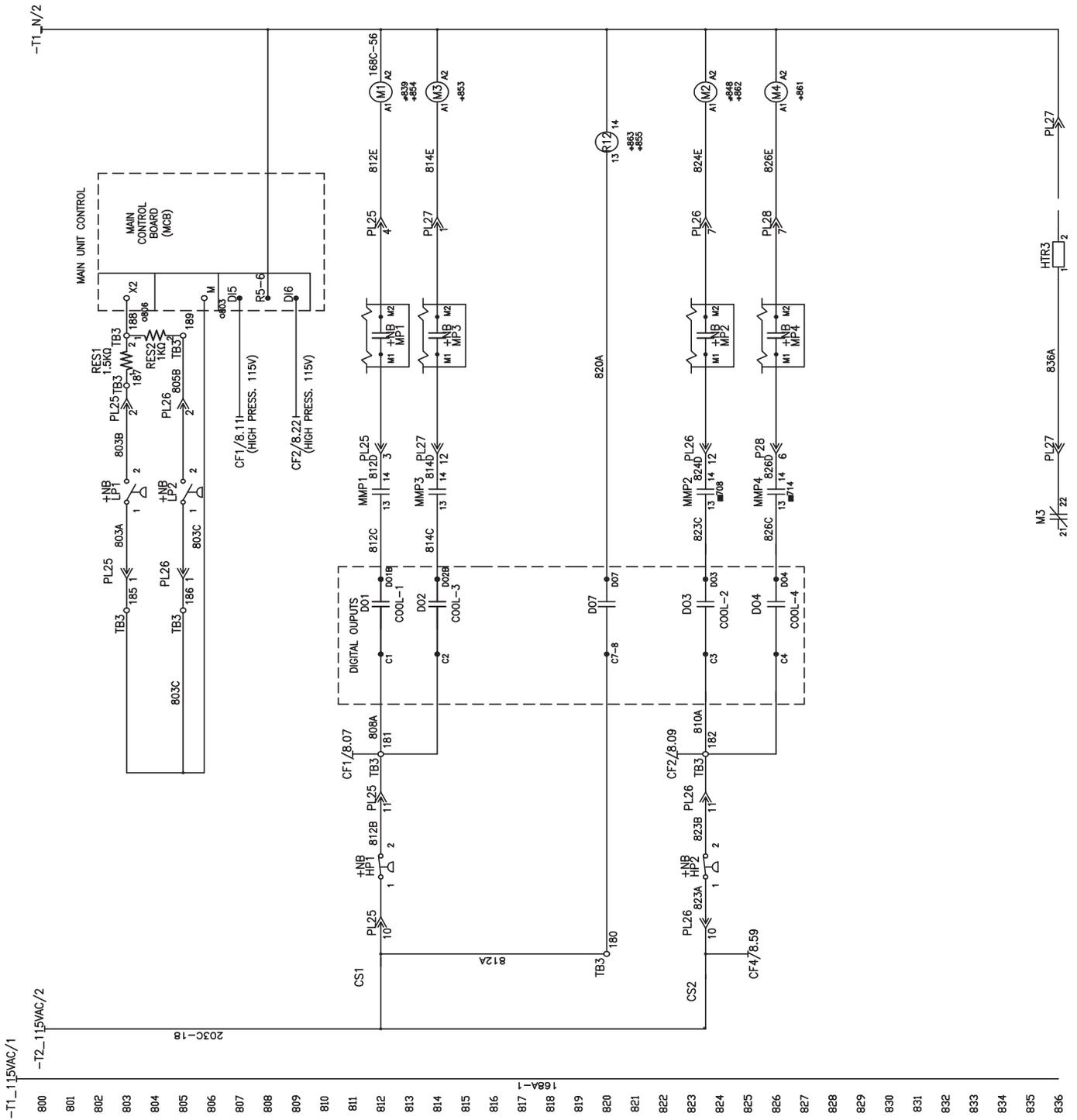
Figure 91 continued: RPS 60 Condensing Unit Control (with Scroll Compressors)
