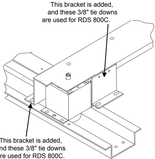
Figure 77: Fan Spring Mount Adjustment
