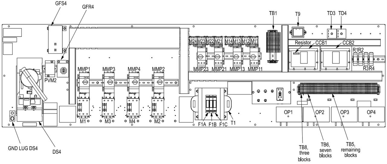
**Figure 22: Electric Heat Panel, Sizes 015C - 040C**
