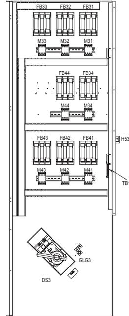
**Figure 23: Electric Heat Panel, Sizes 045C - 075C**
