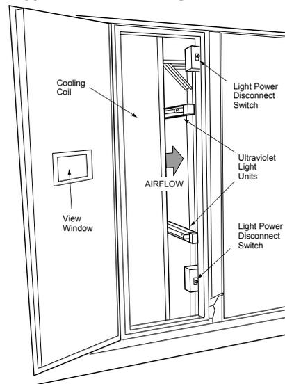
Figure 113: Typical Ultraviolet Light Wiring Schematic
