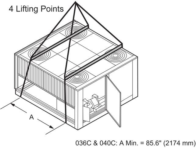
**Figure 41: Unit Type RCS or Condenser Section from RPS/ RDT Factory Split at Condenser**
