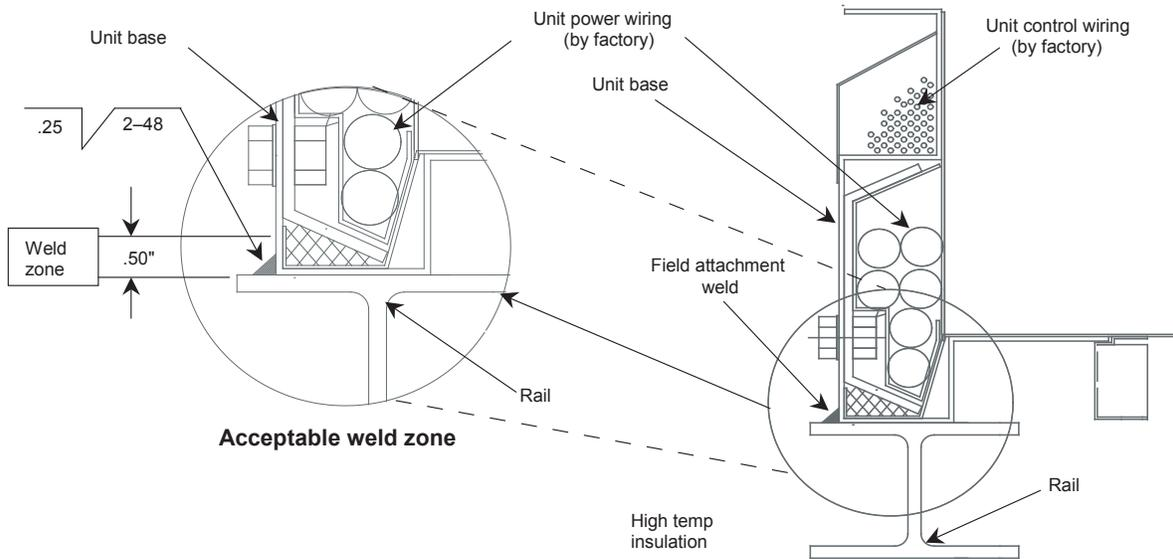
Figure 34: Weld Locations for Rail Arrangement
