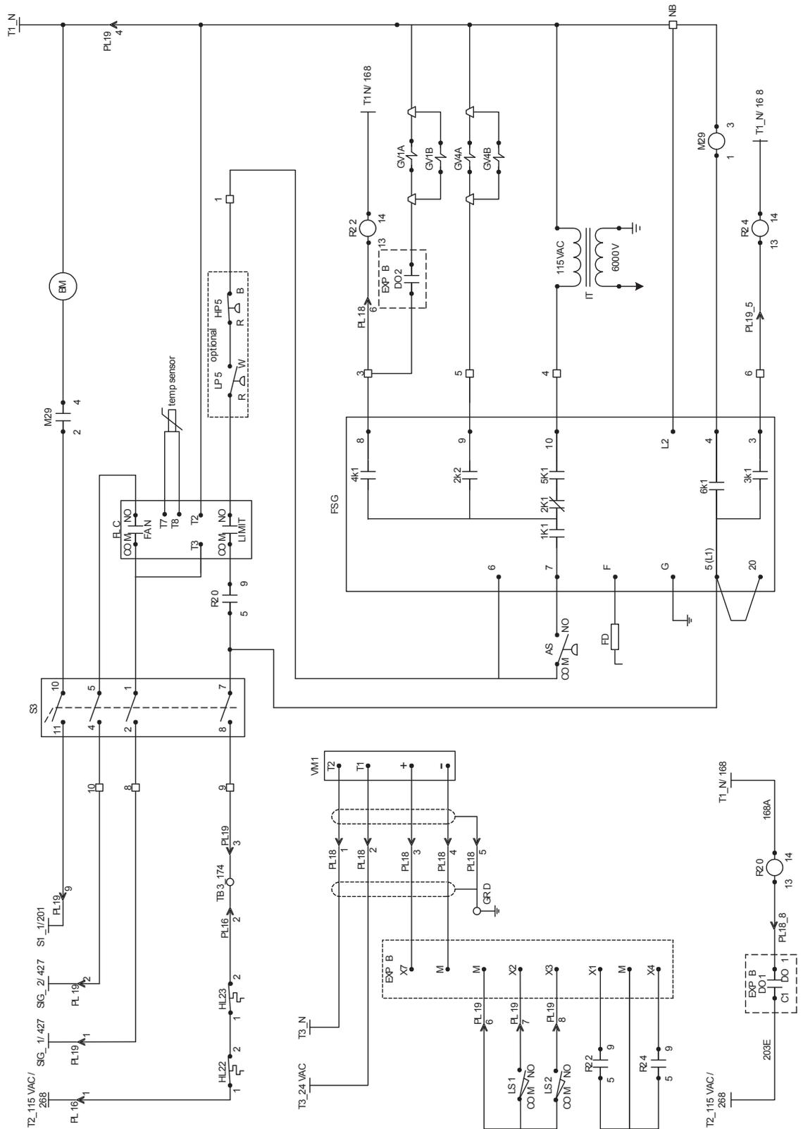
Figure 89 continued: HTD Gas Burner Schematic
