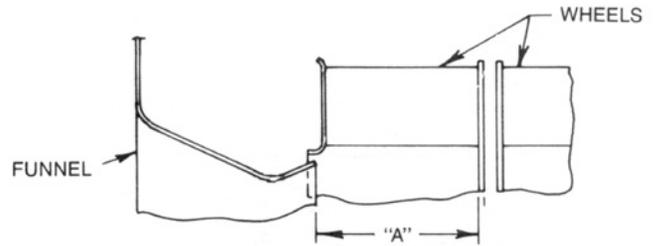
**Figure 125: 40" SWSI Airfoil Wheel-to-Funnel Alignment (RDT 045 to 075)**
