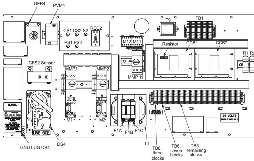
**Figure 20: RCS Control Panel with MicroTech III, RPS 045C - 075C**
