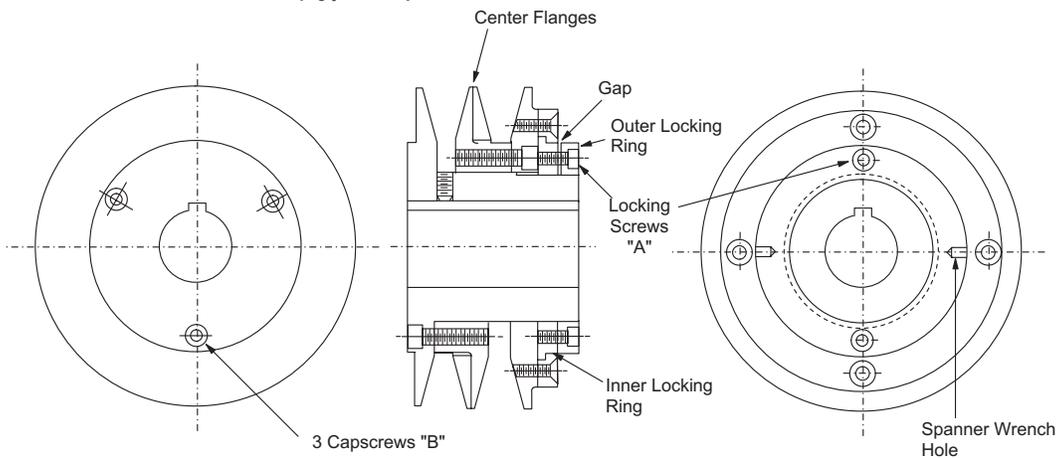
Figure 120: MVP Variable Pitch Sheaves (Type A-B)
