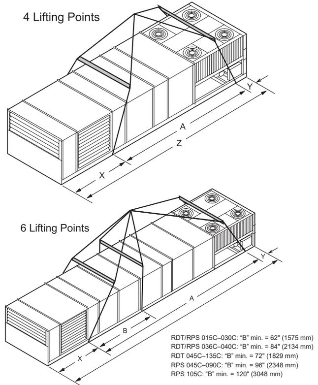
**Figure 39: Unit Type RFS or RPS/RDT Factory Split at Condenser**
