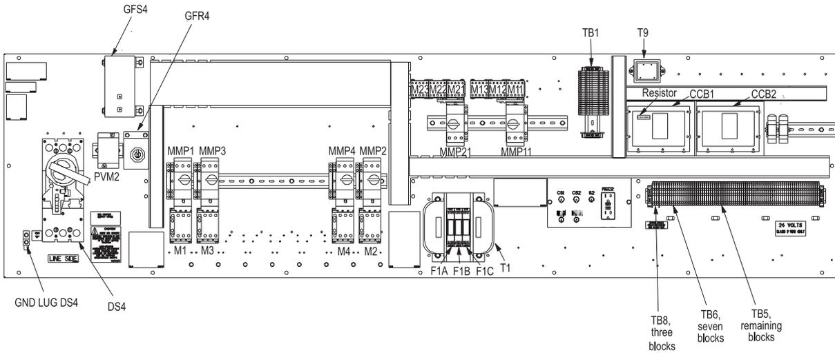
**Figure 21: RCS Control Panel with MicroTech III, RPS 080C - 105C**
