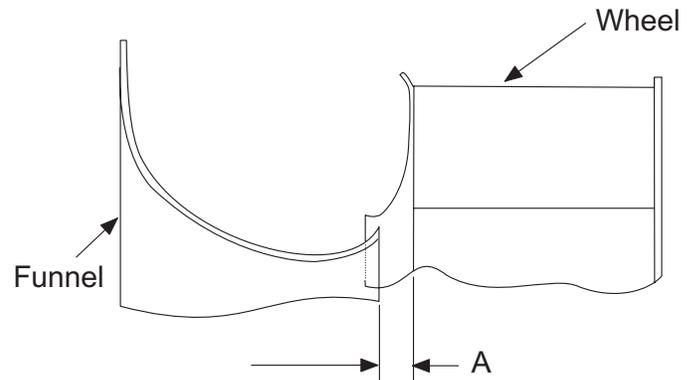
**Figure 126: 44" and 49" SWSI airfoil Wheel-to-Funnel Alignment**
