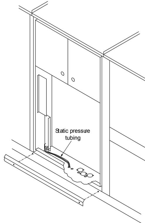
**Figure 66: Pressure Sensing Tubing Installation**
