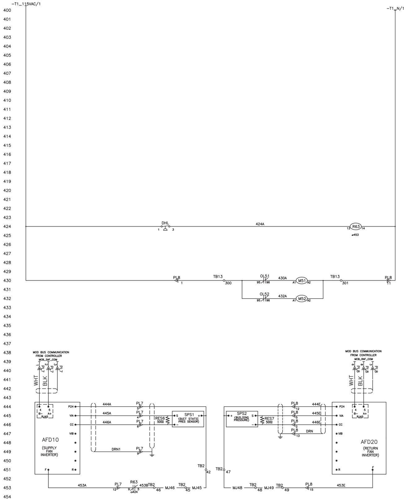
Figure 88: VAV Control Inputs
