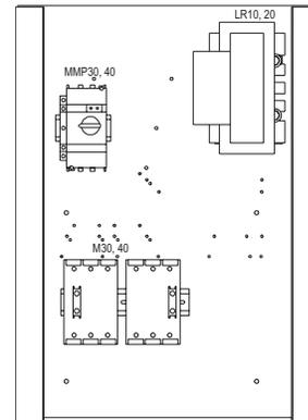
**Figure 19: RCS Control Panel with MicroTech III, 015C - 040C**
