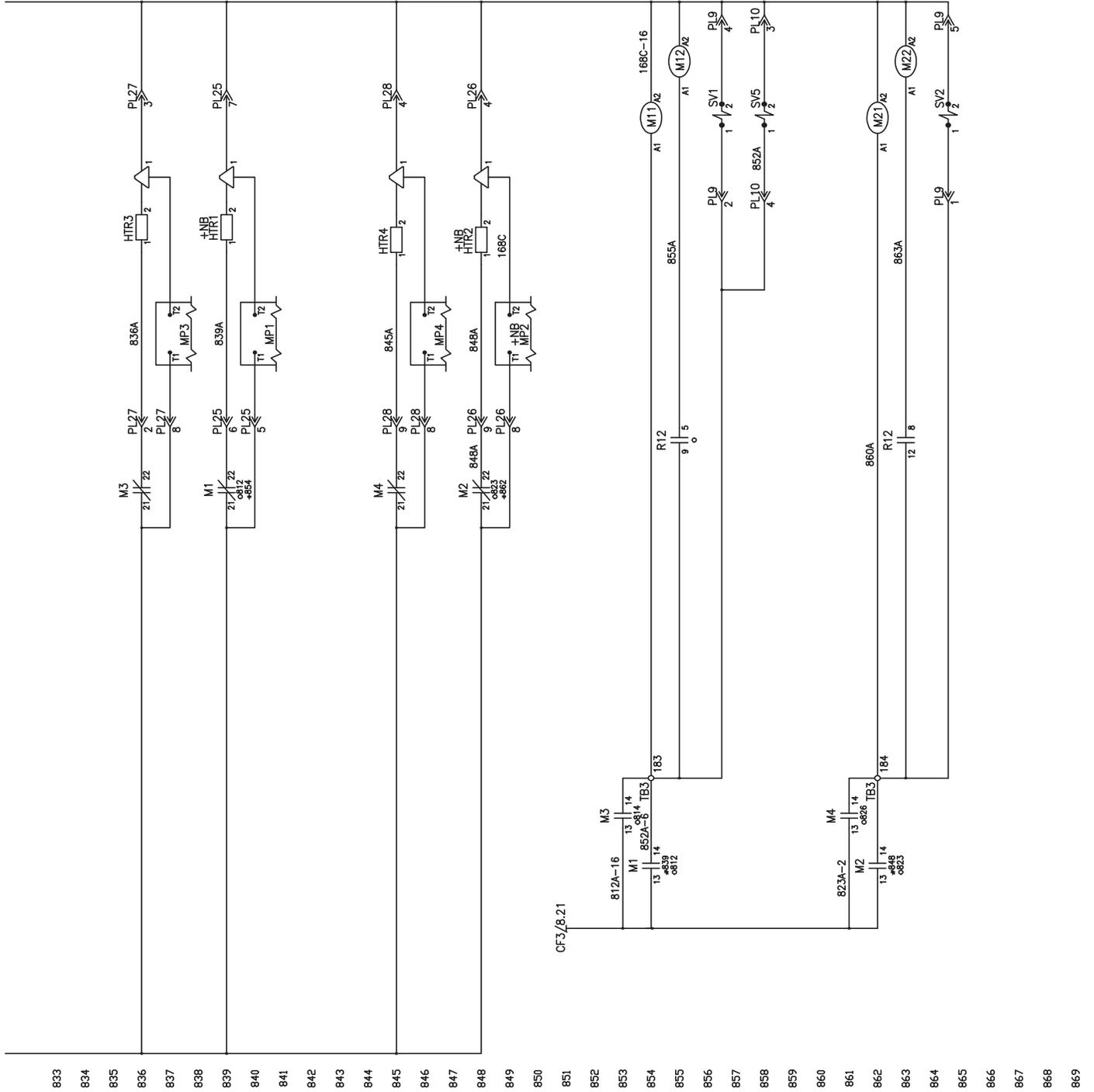
**Figure 92: CV Fan Control (SAF and RAF)**
