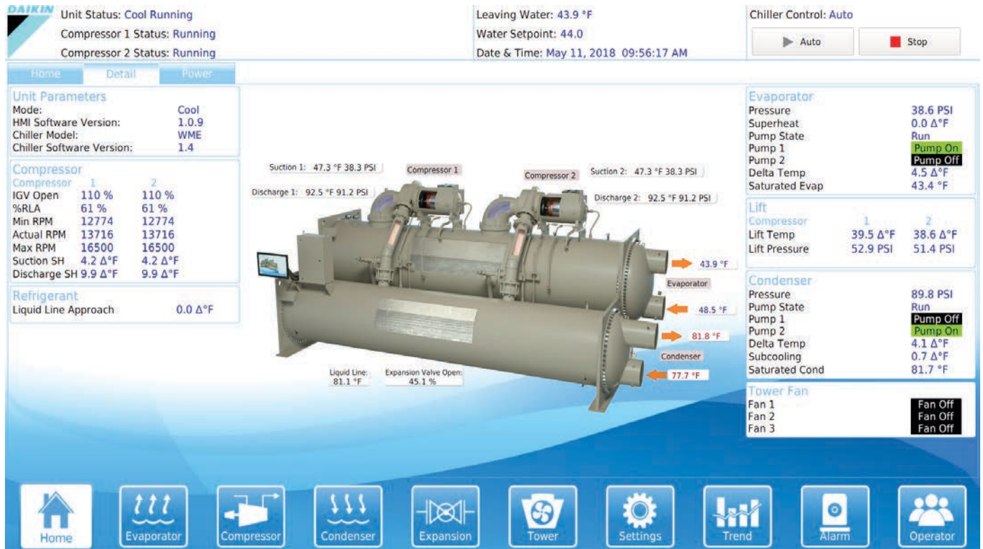
Figure 27: Unit Detail View Screen
