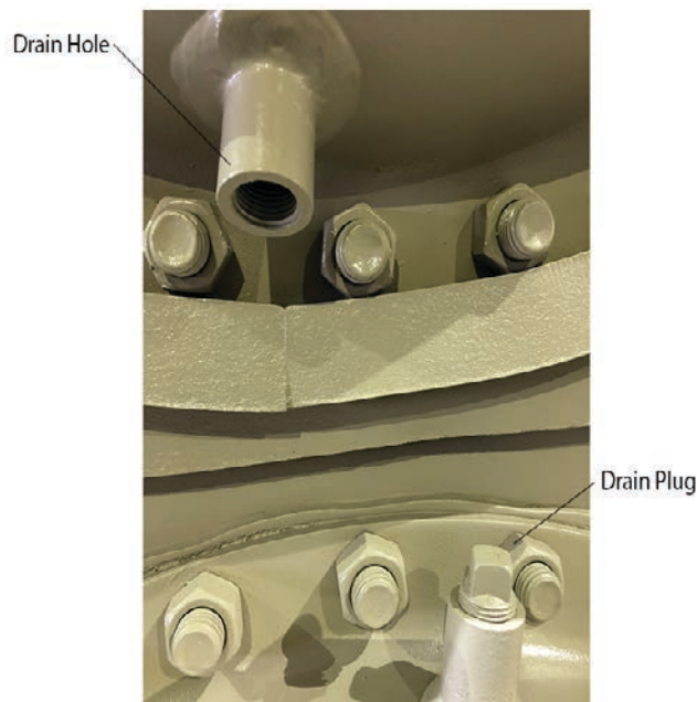
Figure 15: Drain Plug Installation
