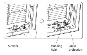
② Lift the air filter and unhook the hooking hole of the air filter from the projection at the grille upper part. (both left and right)
