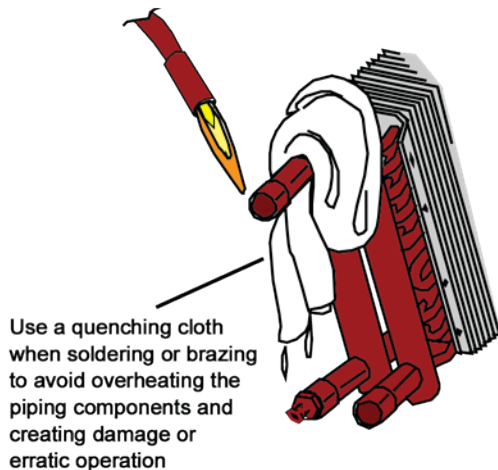
Figure 6: Protect Components from Overheating
