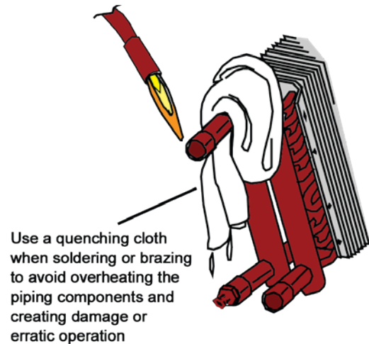
Figure 7: Protect Components From Overheating
