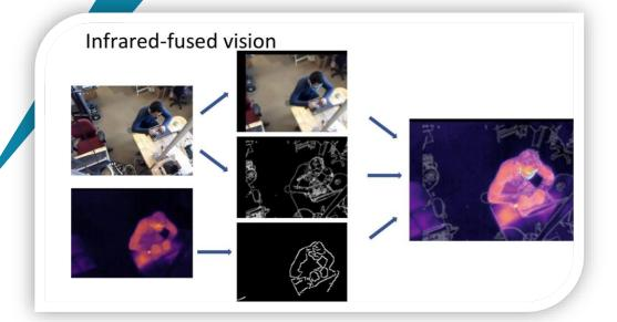
Our method of Thermal image processing uses patented Al technology for generating Infrared Fused Vision where we can overlay a normal image over an infrared image to detect the body temperature and people recognition in the same field of view. Software also includes on-screen and audible alerts to identify one or more individuals in a screening situation with visible temperature tracking, aiding rapid detection and maintaining pedestrian flow.
