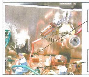
Install a wire from the base of the MRF455 to the left hole of L38.
