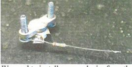
We need to install a ground wire from the mounting screw to the Emitter tabs on the final. I just use the stiff wire found on a resister bent in a U shape to go around the mounting screw.
