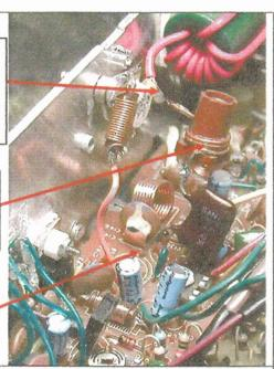
Almost forgot. Because the chassis is originally floating ground the radio has to be modified to give a DC Electrical ground to the final (Mounted on the Floating Chassis Ground).
