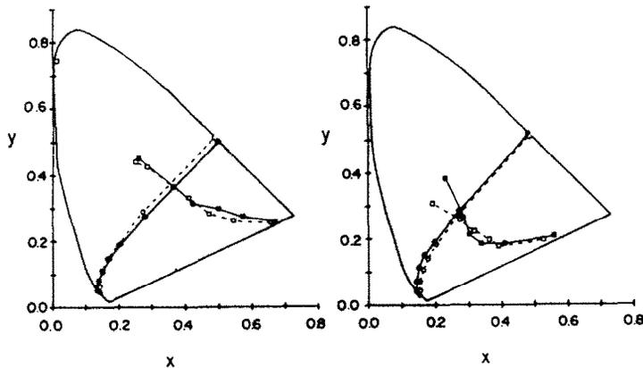
Fig. 5. Comparison of unique hues generated for the 2 deg (solid lines) and 40 min (dashed lines) conditions: observers as above. Unique blues and yellows were determined by mixing various proportions of each observer's unique yellow and a variable short wavelength light. Unique red and green loci were determined using a three primary method.
