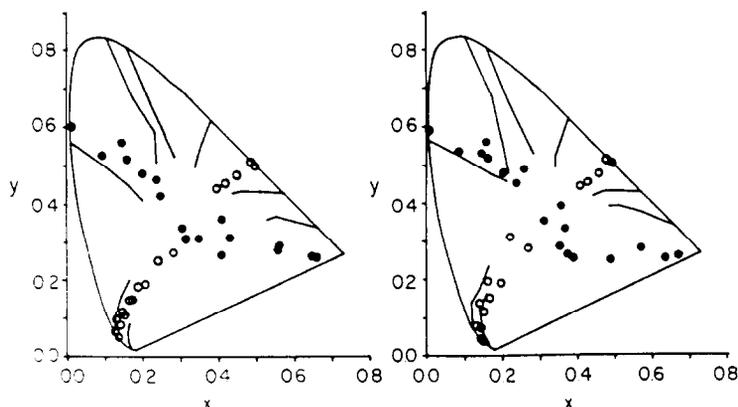
Fig. 6. Summary of constant hue data plotted in the Judd (1951a) chromaticity diagram: observers as above. Solid lines—data from hue matching at 0.54 c/deg; open symbols—unique yellows (white desaturant) or unique blues (white and unique yellow desaturants); closed symbols—unique reds and greens (spectral and two-primary data).
