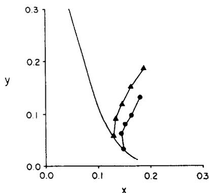
Fig. 3. Comparison of unique blue loci for observer S.B. using a double random staircase technique (circles) and the method of adjustment (triangles). The desaturant was 571 nm for both experiments. Data were collected about 3 months apart.
