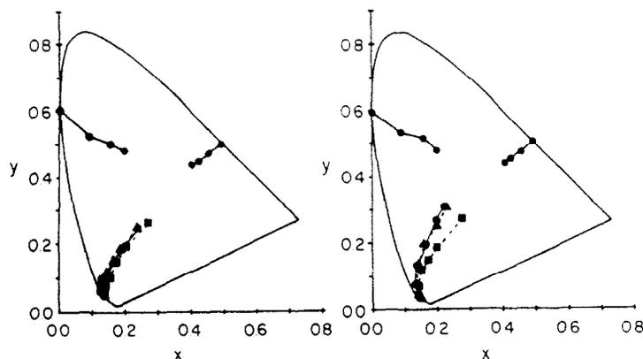
Fig. 2. Unique blue, green and yellow loci plotted in the Judd (1951a) chromaticity diagram: observers as above. Unique hues were obtained as mixtures of white and monochromatic lights (circles and solid lines), as mixtures of unique yellow and monochromatic lights (squares and dashed lines), or as mixtures of a 571 nm light and monochromatic lights (triangles and dashed lines).
