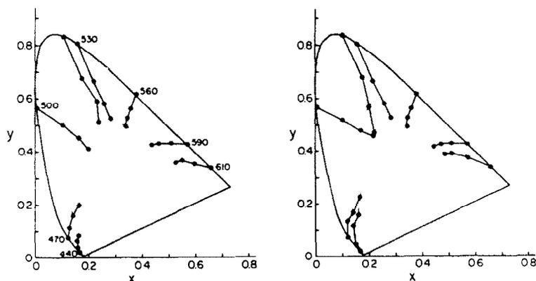
Fig. 1. Constant hue loci plotted in the Judd (1951a) chromaticity diagram: observer S.B. left, A.E. right. Error bars indicate confidence intervals of 2 SEM around the mean. For data with no error bars, either the confidence interval was less than 1 nm, or too small to be seen on the figures.
