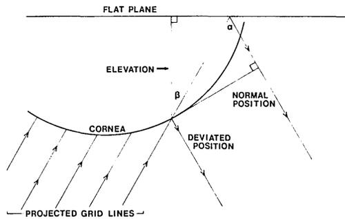
Fig. 5. Schematic diagram showing grid lines displaced on cornea from assumed normal position and trigonometric solution for elevation.
