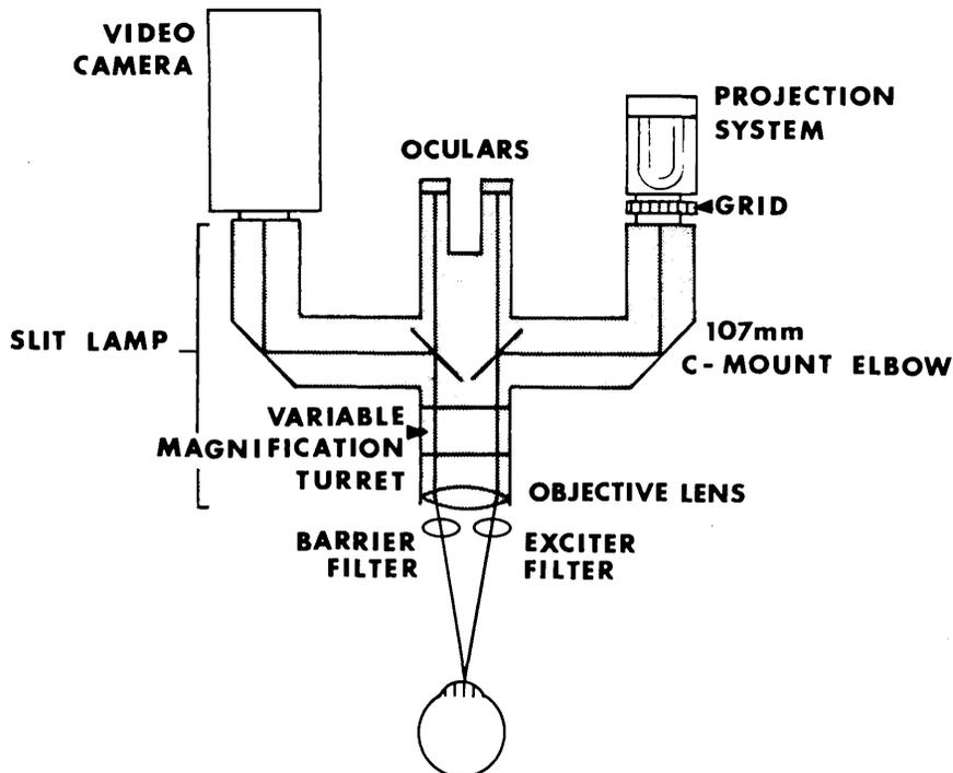
Fig. 3. Schematic diagram of Zeiss microscope with beam splitter and projection system attached.
