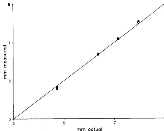
Fig. 10. Graph comparing grid curvature measurements with micrometer readings; four points plotted for each steel ball.
