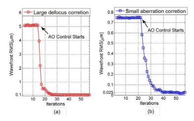
Fig.3. Wavefront error reductions of (a) large and (b) small aberrations over a  $\Phi$ 7.56mm pupil
