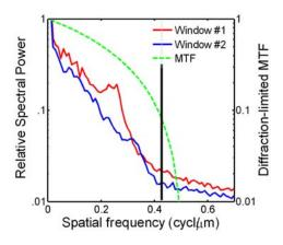
Fig. 10. Left: Image of subject S4. Right: Power spectrum of the two windows indicated on the left. Curves are the total power at a given frequency over all orientations. For reference the diffraction-limited MTF of a system with the same numerical aperture is shown in green curve and the vertical black line shows Rayleigh diffraction limit, which is 0.42 cycle/ $\mu m$  in this figure for pupil size of  $\Phi 7.2$  mm.
