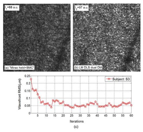
Fig. 7. Retinal images obtained with (a) successive dual DM AO and (b) simultaneous LM DLS dual DM AO. (c) Wavefront error reduction with the DLS AO routine correction (Pupil size 6.48mm)
