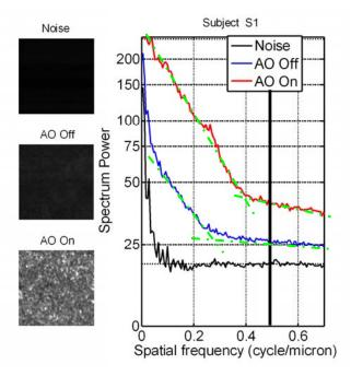
Fig.8. Comparison of noise (no eye in system), foveal images with and without AO
