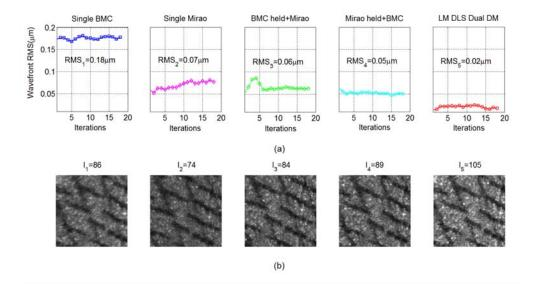
Fig.4. Comparison of wavefront control between different AO modes.
