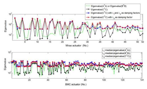
Fig. 2. Eigenvalues spectrum conditioning for the normal control matrices Top panel: Eigenvalues of the Mirao DM. Bottom panel: Eigenvalues of the BMC DM.
