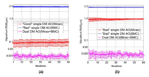
Fig. 5. Comparison of wavefront control accuracies of a single DM AO (Mirao, and BMC) with the LM DLS dual DM AO (Mirao+BMC): (a) "Well-calibrated" Mirao DM + "Badly-calibrated" BMC DM. (b) "Badly-calibrated" Mirao DM + "Badly-calibrated" BMC DM.
