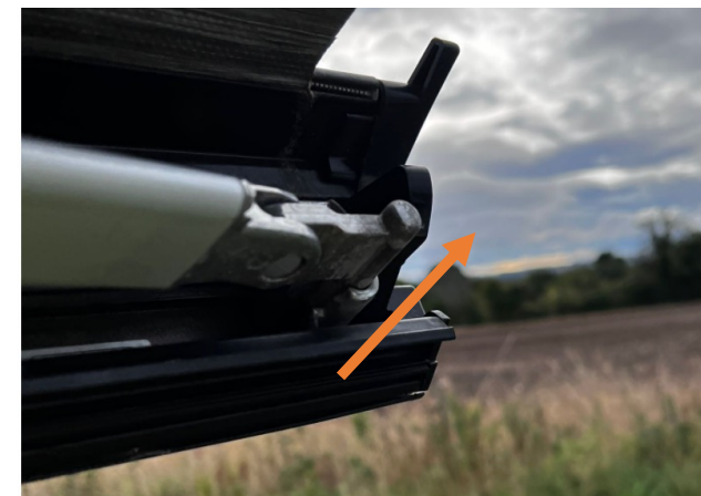
Pull pivot pin on corner towards you, this will allow leg to swing down
