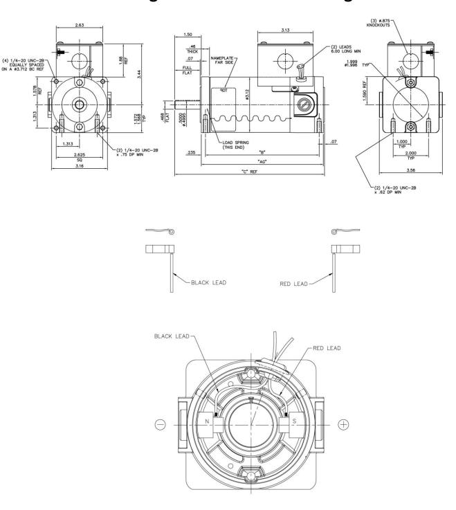
EXTERNAL CONNECTIONS FOR CCW ROTATION VIEWING LEAD END OF MOTOR WITH RED LEAD POSITIVE (+) AND BLACK LEAD NEGATIVE (-). FOR CW ROTATION REVERSE POLARITY.
