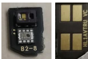
Figure 6-1 Proximity sensor sub-board
