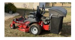
The Ferris. The zero-turn mower with bagger attachment. Used during the regular mowing season and assists with leaf cleanup.
