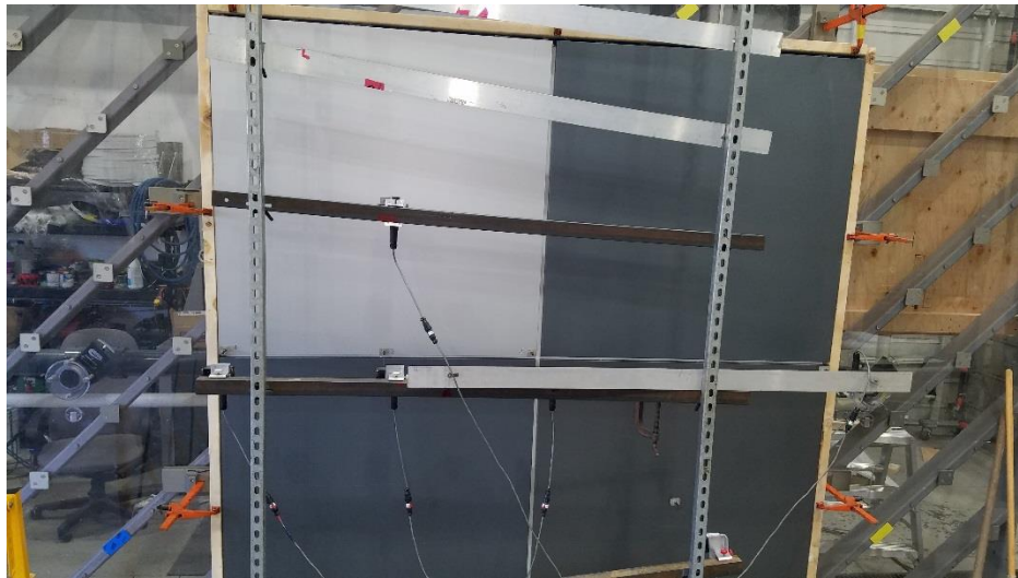
Photo No. 5 Test setup – Uniform Load Test
