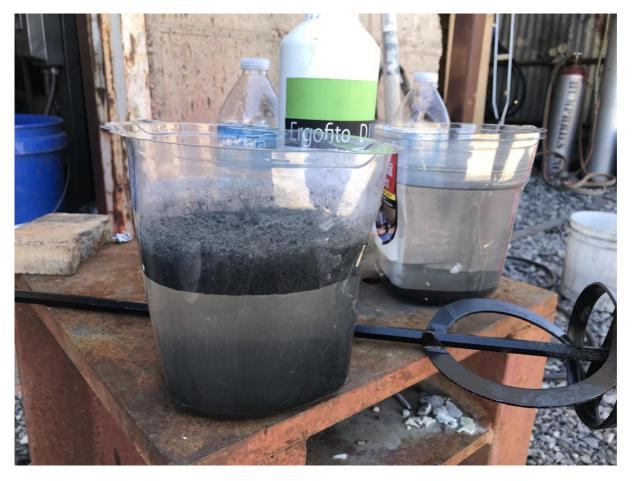
The above two containers demonstrates the oil separation. Oil contaminated sludge with water and Ergofito Dil are put into a container.
