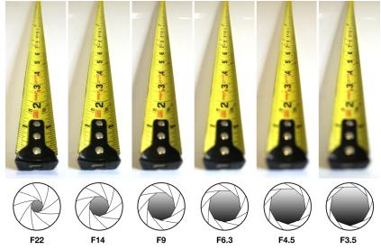
Notice the ruler is completely in focus on the left with the F16 setting, yet the ruler on the far right only has one point in focus with an F1.4 setting.
