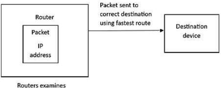
packet to look for header that has the IP address of destination
