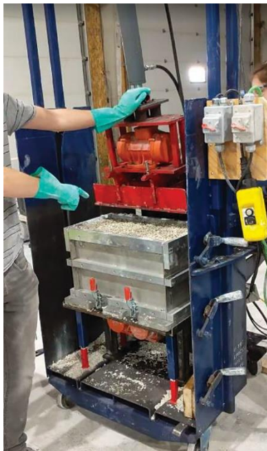
Figure 4 • Manually clamped and externally vibrated individual hempcrete block mold prototype. Reproduced with permission from ClimatBloc [42].
