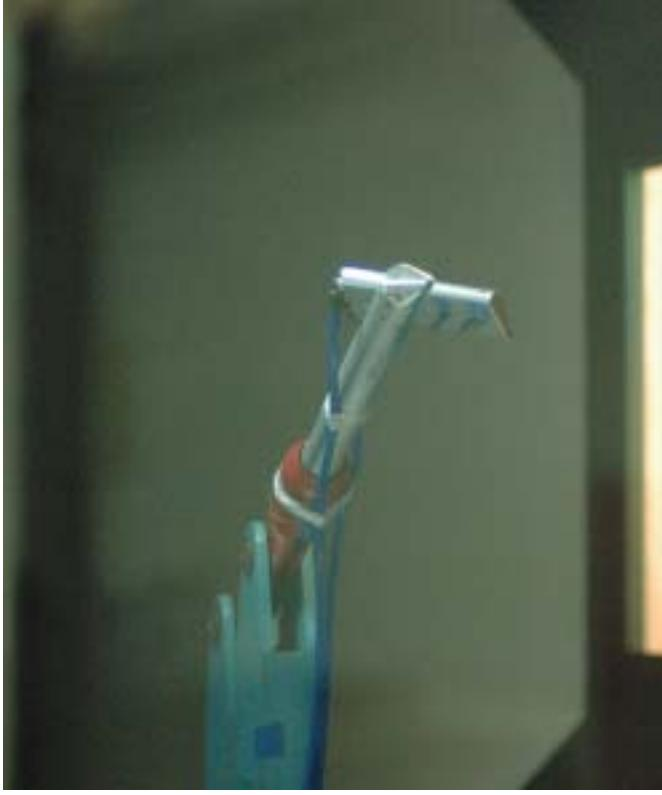
**Figure 13.** Angle of attack probe pitched 25°, yawed 10° and rolled 45°.
