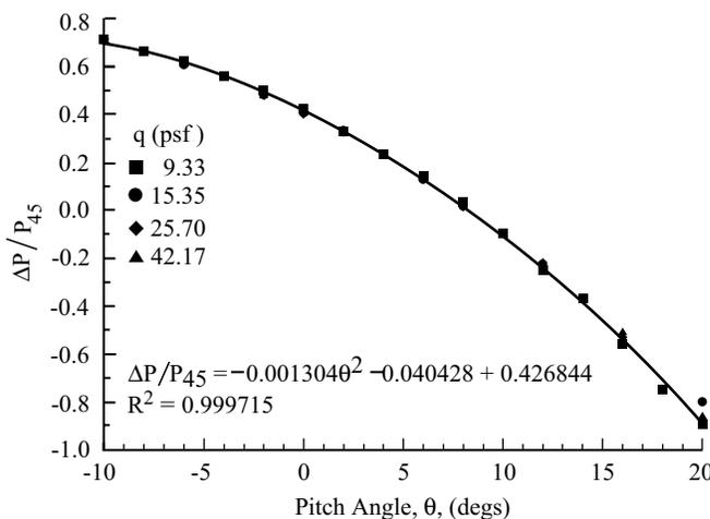
**Figure 11.** Alternate method of normalizing the differential pressure.
