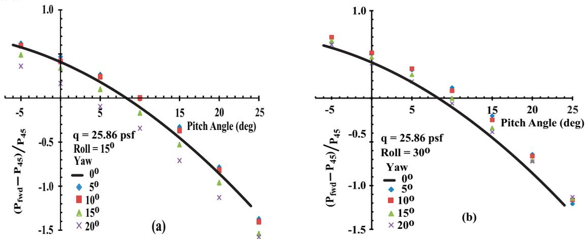
**Figure 16.** Effect of combine pitch, yaw and roll on the normalized differential pressure for a dynamic pressure of  $25.86 \text{ psf} \approx 100 \text{ MIAS}$ ; (a) roll =  $15^\circ$ , (b) =  $30^\circ$
