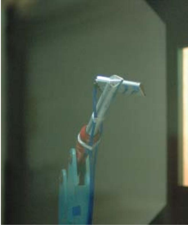
**Figure 13.** Angle of attack probe pitched  $25^\circ$ , yawed  $10^\circ$  and rolled  $45^\circ$ .
