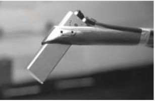
Figure 3. Angle of attack probe mounted in the wind tunnel.
