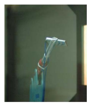
Figure 13. Angle of attack probe pitched 25°, yawed 10° and rolled 45°. The viewpoint is directly into the image.
