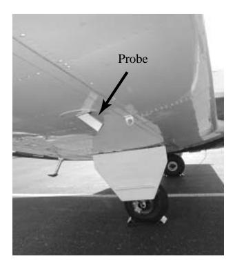
Figure 1. Angle of attack probe mounted under the wing.
