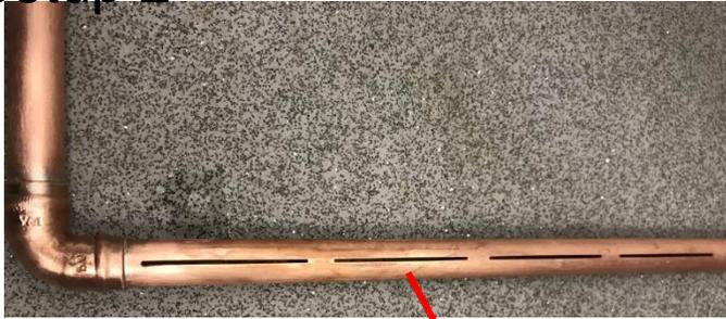
Thin (1mm) slits used to extract at specific vertical height
