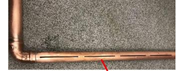
Thin (1mm) silts used to extract at specific vertical height
