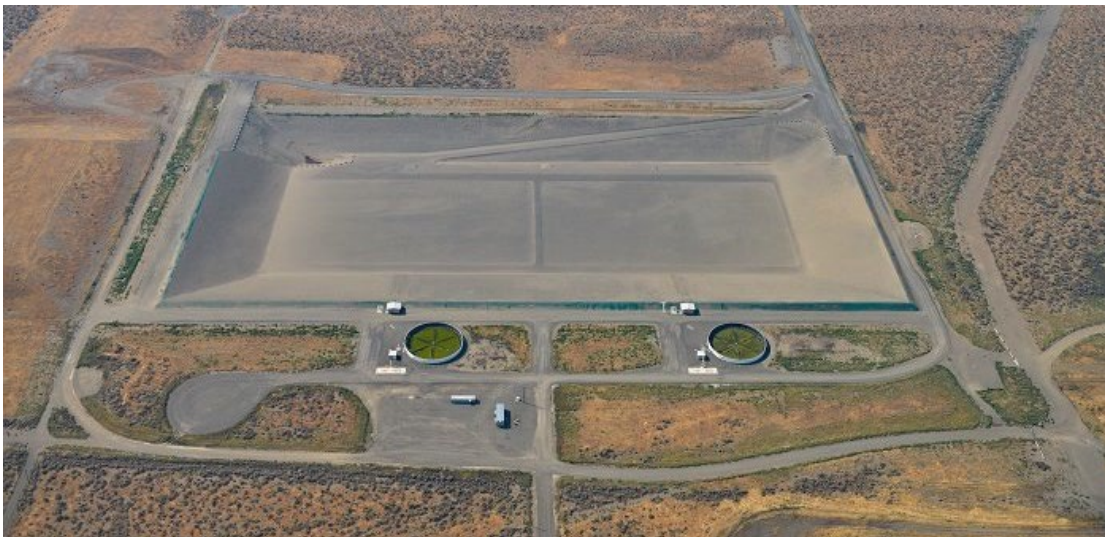
Hanford's Integrated Disposal Facility, an engineered disposal site designed to receive immobilized low-activity waste from the WTP and MLLW from Hanford Site operations
