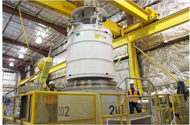
INL Advanced Mixed Waste Treatment Project crews prepare a transportation cask containing TRU waste for shipment to WIPP.
