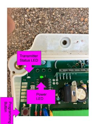
Pre Req: Have Remote in one hand and the other hand ready to press button on receiver in gatewise module.
