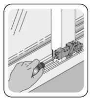
You can adjust your patio door rollers by inserting a Phillips screwdriver through the hole located at the lower end of each door vent panel and at all four corners of your screen door.
