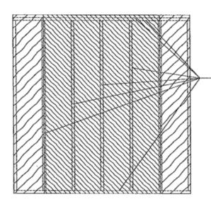
Use a minimum 1 1/2 inch long drywall screws, nails or staples at 6 inches on center along the panel edge and 12 inches on center in the field to the framing members. It is particularly important to pay attention to these details at the top and bottom of the applied panel.
