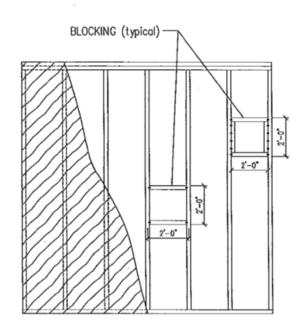
Damaged Wall board "patch" material shall be an equivalent thickness of gypsum
