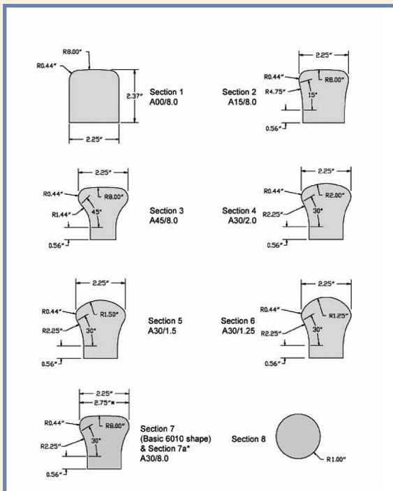
Many handrail shapes were considered: Round plus milled with a width between 2 1/4 and 2 3/4 in. and a crown radius between 1 1/4 and 8 inches, with varying recesses on the sides.
