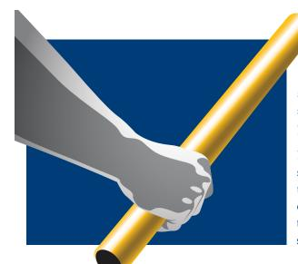
Decades ago, a study of just 20 subjects changed the face of the stair industry. While restrained in a standing position, pushing and pulling forces on a handrail were measured and the subjects' opinions recorded. This lead to the conclusion that a certain round shape, among those tested, provided a grasping surface against which subjects generally could generate high pushing and pulling forces.
