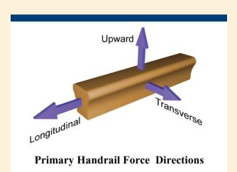
The study indicated that subjects both pulled upward and pushed downward on the handrails. Transverse forces were inward pulls, not outward pushes. In the longitudinal direction, test subjects were pulling on the handrail, meaning that their bodies were even with or ahead of their grasping hands when they exerted the peak forces. When they exerted the peak forces, their bodies were lowered, with their arm outstretched.
