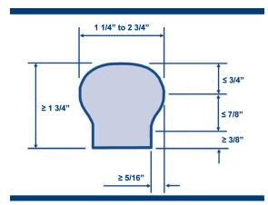
On the basis of the tests and comparisons, it was proven that the influence of crown height and handrail width are minimal for the shapes that were examined. Further, it was concluded that the depth of recess defined by a sweep angle of 30 degrees provided graspability that is comparable to that of a 2 in. round handrail.
