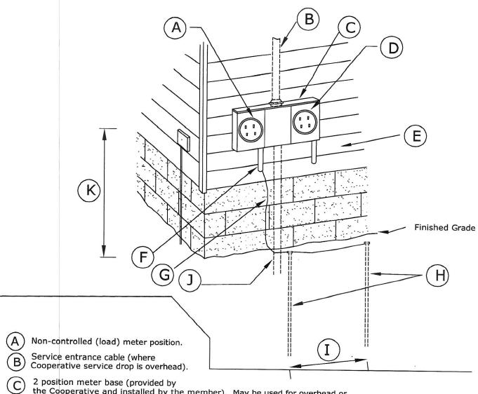
the Cooperative and installed by the member). May be used for overhead or underground service drops.
