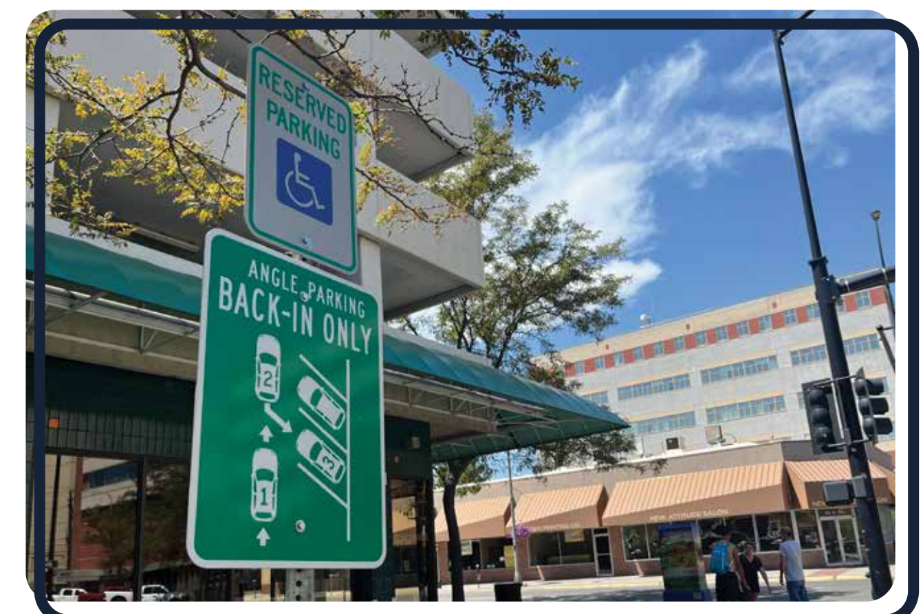
Back-in angle parking can also lower the risk of collision with bicyclists and pedestrians and provide a safer experience for passengers when entering and exiting a vehicle.
