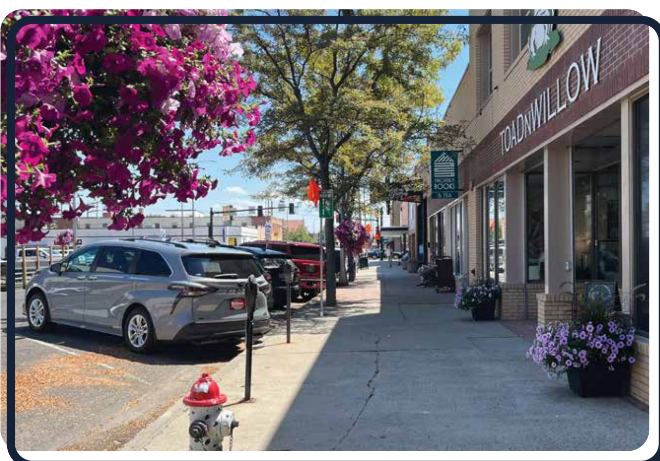
Safety benefits of back-in angle parking include more visibility when exiting the parking spot and safer unloading/loading from the sidewalk.
