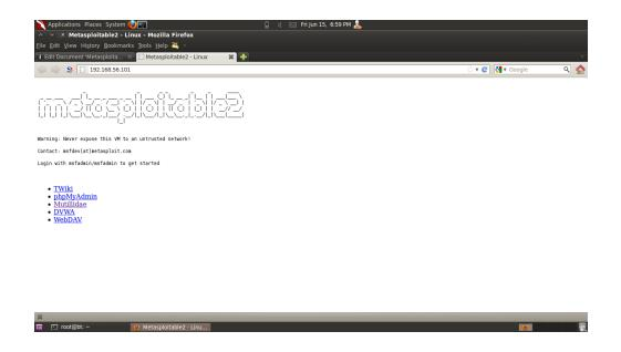
192.168.56/24 is the default "host only" network in Virtual Box. IP address are assigned starting from "101". Depending on the order in which guest operating systems are started, the IP address of Metasploitable 2 will vary.
