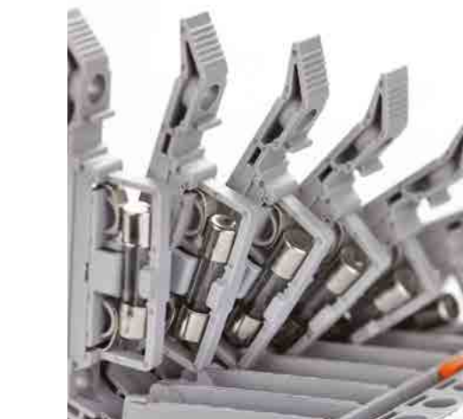
Screw Connection Fuse Rail Terminals Terminals can be used with glass fuse between 1A...10A. The fuse inside of the terminal is easily mounted and dismantled, and is an ideal solution when there is a necessity to change it even when the power is on in the system. Marking solutions can be provided by Plotter Labeling.
