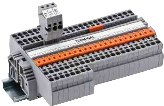
PYK series Disconnect Terminals enables to safely open-close the circuit , when the energy is on in the system. Can be marked with Thermal marking strip and cross-connected together with all other single-level terminals. Special Marking solutions can be provided by Thermal Printing and Plotter Labeling.
