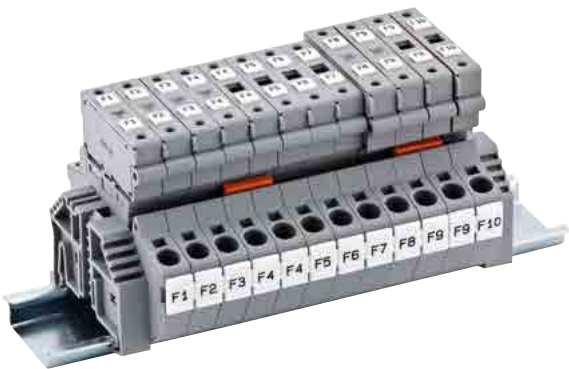
Practical Spring Clamp Fuse Terminals has a sliding type hinged carrier that has a specially designed space for cartridge type glass fuse of size Ø 5x20 or Ø 5x25 together with a spare one. Both sides of the terminals are closed and available for cross connection. Special Marking solutions can be provided by Plotter Labeling.
