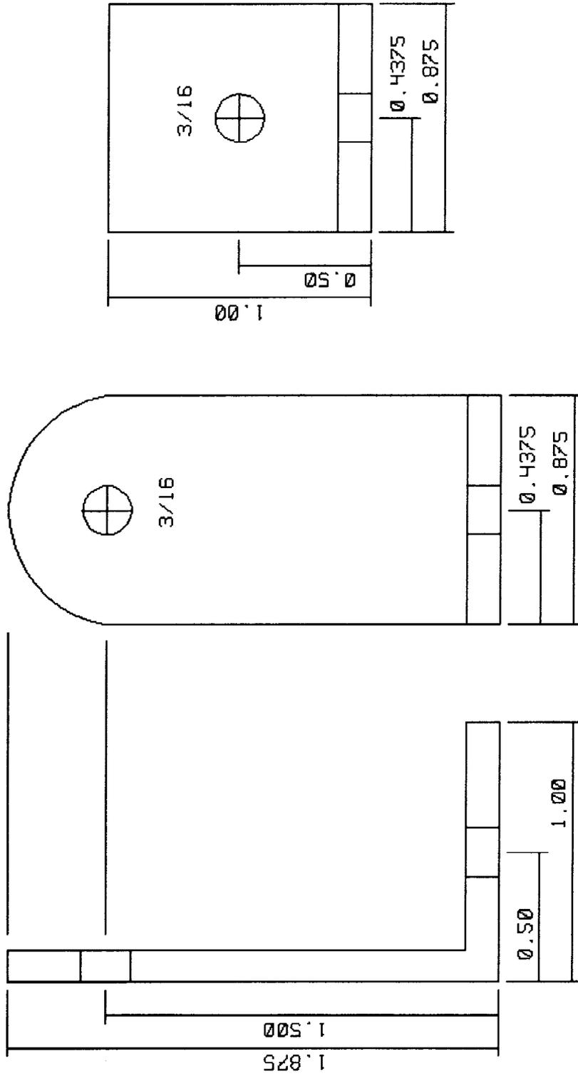
FABRICATE BRACKETS FROM PIECES CUT FROM 2 X 2 X 1/8 INCH SQUARE EXTRUDED ALUM. TUBE STOCK
