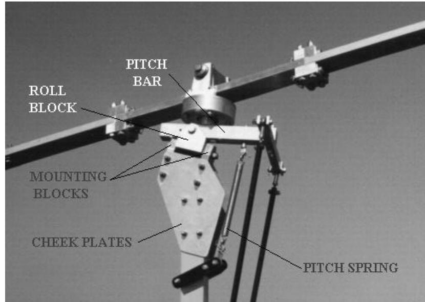
Shown above is a nice photo of the *Gyrobee* head assembly made during our first flying season. I have labeled the critical parts to make it easier to make sense of the discussion which follows.
