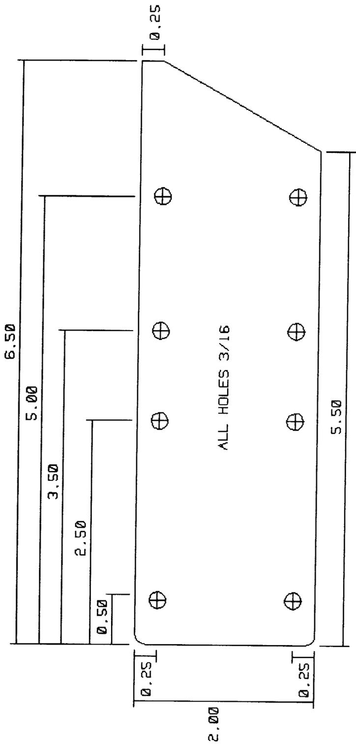
NOSE BLOCK CHEEK PLATES (2 ROD) - 1/8 INCH 6061-T6 SHEET.
