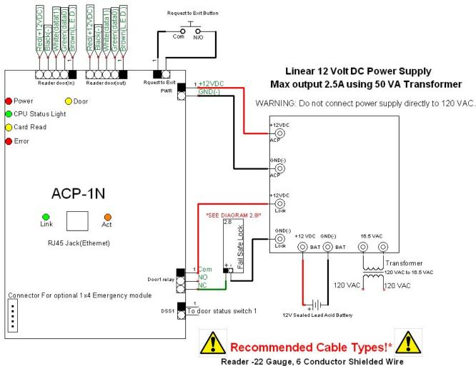
Locking Hardware- 18 Gauge or better, 4 or 6 Conductor Wire \*use of other cabled types such as CAT5 for these devices may void your warranty.
