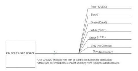
EACH READER HAS A SHIELDED CABLE. CONNECT SHIELD TO SHIELD AT THE CARD READER. CONNECT SHIELD TO GROUND (-) AT THE CONTROL PANEL INPUT FOR EACH INDIVIDUAL READER. Use 22awg 5 conductor or better stranded cable with an overall shield for proximity reader wiring.
