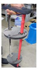
The rods and plates are titanium. Contacting water with these electrified plates generates the nano-bubbles. A lot of it! there is no need for pH adjustment such as KOH.
