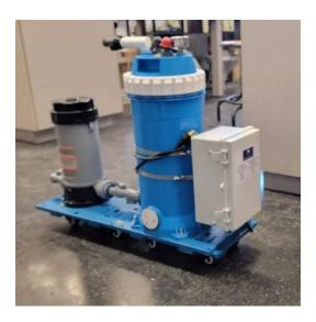
The Nano-Bubble maker is composed of 2 housing filters. The Grey one-or-first filter housing is for <u>Citric acid powder</u> or <u>descaling powder</u>. It's typically set at 0 as we do not need it until there's a problem with the blue reactor plates. Scaling plates depends on the hardness of the water. Thus, using the descaler could be needed once a month or once a week. Water softeners ahead of our technology do help.
