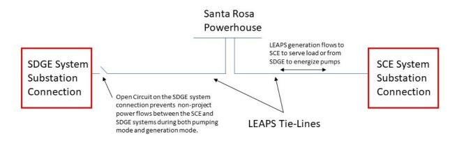
Configuring LEAPS with circuit breakers and switches to ensure that only one connection is "open" at any time guarantees that all facilities operate as "project primary" facilities which carry only LEAPS power. Unlike the LEAPS project configuration proposed by TNHC, this "open" configuration properly complies with the FPA; it is also considerably cheaper because it does not include costly phase shifters.
