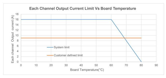
The end user can define the input power and output current limit. The final value depends on the temperature and will always take the lower of the user defined limit and the system limit.
