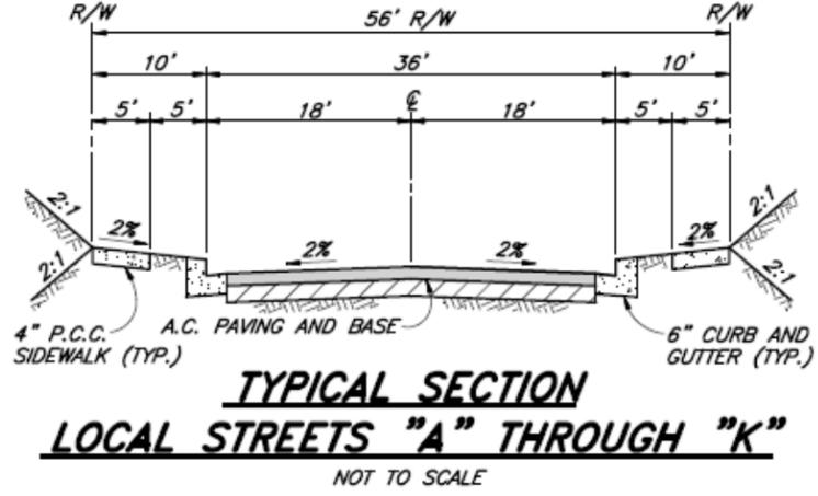
See Figure IV-66 for Plan View and Section
