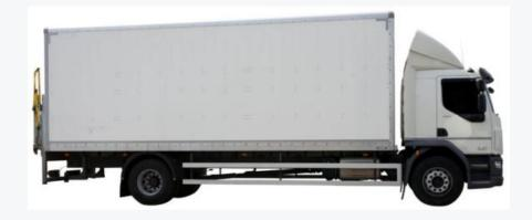
These trucks have a lifting mechanism so as to load goods onto the truck. These are relatively small in size ending upon the tail lift it can carry a maximum of 2000 kg. The goods can be loaded only from the back side and is used mainly on distribution freights.
