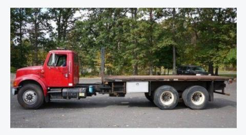
These trucks are named so as it has an open cargo bed trailer along with the driver's cabin. As flatbed trucks don't have a roof or sides it is easy to load or unload goods on or from it.
