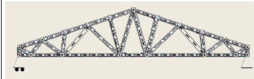
**Annealed** : lower chord 100x60x4, upper chord 80x80x5, corner vertical 60x60x5 diagonals from left to middle: 50x50x3, 50x50x3, 40x40x3, 40x40x3, 40x40x3, 40x40x3, 40x40x3, 40x40x3.
