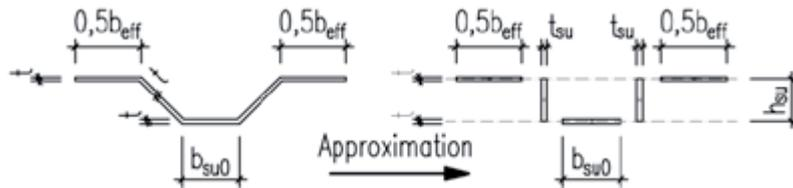
$$t_{\text{su}} = \frac{\sqrt{h_{\text{su}}^2 + \left(\frac{b_{\text{su}} - b_{\text{su}0}}{2}\right)^2}}{h_{\text{su}}} t = \frac{\sqrt{6^2 + \left(\frac{20 - 8}{2}\right)^2}}{6} \times 0,6 = 0,849 \text{ mm}$$
