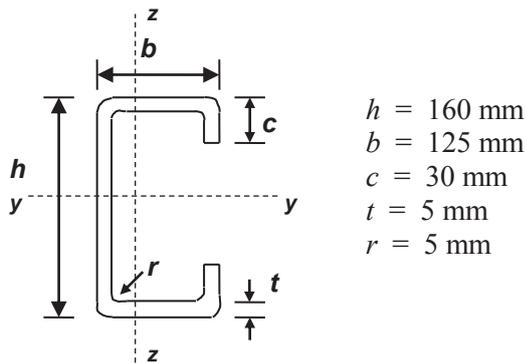
$$\begin{aligned} h &= 160 \text{ mm} \\ b &= 125 \text{ mm} \\ c &= 30 \text{ mm} \\ t &= 5 \text{ mm} \\ r &= 5 \text{ mm} \end{aligned}$$
